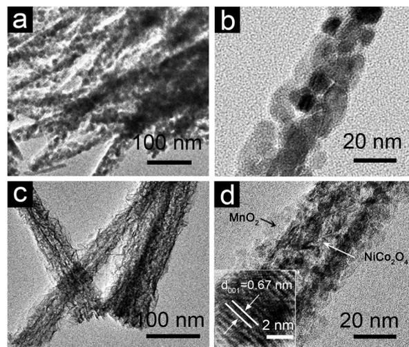
**Fig. 3** TEM images of (a, b)  $\text{NiCo}_2\text{O}_4$  NWs and (c, d)  $\text{NiCo}_2\text{O}_4@\text{MnO}_2$  core-shell heterostructured NWs scratched from Ni foam. The inset of (d) shows a HRTEM image of  $\text{MnO}_2$  nanoflakes.
