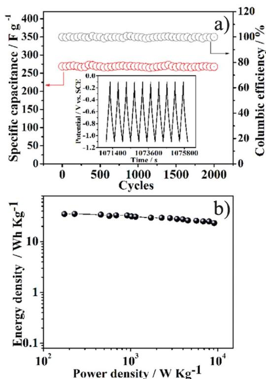
**Fig. 6** a) Variations of specific capacitance and the coulombic efficiency versus the cycle number of NGS-1 measured at a current density of  $1 \text{ A g}^{-1}$  within the potential range from  $-1.1$  to  $-0.1 \text{ V}$ . The inset shows the charge–discharge curves of the last 10 cycles for NGS-1. b) Ragone plots of supercapacitors composed of NGS-1 as positive and negative electrodes in  $6 \text{ M KOH}$  electrolyte.
