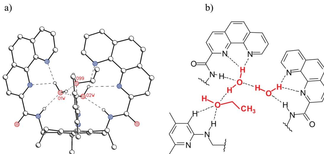
**Fig. 4** (a) Crystal structure of **13** (C-Hs are omitted for clarity); two hydrogen-bonded water molecules and one ethanol molecule are present in the binding pocket of **13**. (b) Schematic representation of the binding motifs in the binding pocket of **13**.<sup>6h</sup>
