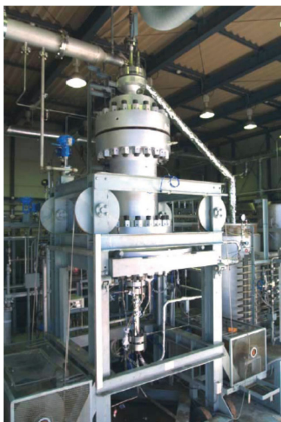
Fig. 20 Industrial supercritical water reactor for organic solvent treatment. This flow reactor can treat 1 metric tonnes waste per day. (The photograph was kindly provided by Organo Corporation (Tokyo). Permission for use was obtained from the company).
