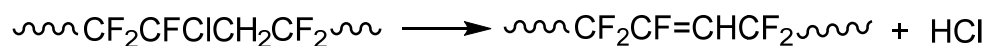
Scheme 9 Thermal degradation of poly(CTFE- co -VDF) copolymer 95 (reproduced with permission from Elsevier).
