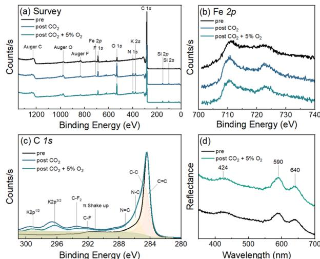
Fig. 7 (a) Survey XPS spectrum, high resolution (b) Fe 2p and (c) C 1s spectra and (d) UV-vis spectra of (FeDVPP)<sub>2</sub>O modified CNT/CP electrodes before and after anaerobic and aerobic (5% O<sub>2</sub>) CO<sub>2</sub>RRs.
