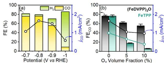
Fig. 5 (a) Faradaic efficiency (FE) and CO partial current density ( $j_{CO}$ ) of heterogenized **(FeDVPP)<sub>2</sub>O** on the CNT/CP electrode in CO<sub>2</sub>-saturated 0.5 M KHCO<sub>3</sub> after 30 min of electrolysis at different potentials. (b) Comparison of performance of **(FeDVPP)<sub>2</sub>O** and **FeTPP** after 30 min of electrolysis at -0.8 V *vs.* RHE at different O<sub>2</sub> volume fractions (in the CO<sub>2</sub> + O<sub>2</sub> mixture).
