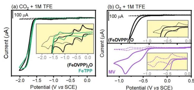
Fig. 3 Cyclic voltammograms of  $0.25 \text{ mM } (\text{FeDVPP})_2\text{O}$  (black) in DMF with  $0.1 \text{ M } [\text{Bu}_4\text{N}]\text{PF}_6$  and  $1 \text{ M}$  trifluoroethanol (TFE) under (a)  $\text{CO}_2$  and (b)  $\text{O}_2$ , in comparison to  $0.5 \text{ mM } \text{FeTPP}$  (green) and  $0.5 \text{ mM } \text{MV}$  (purple). Dotted curves show CV curves recorded in  $\text{Ar}$ -saturated DMF. Insets show zoomed data.
