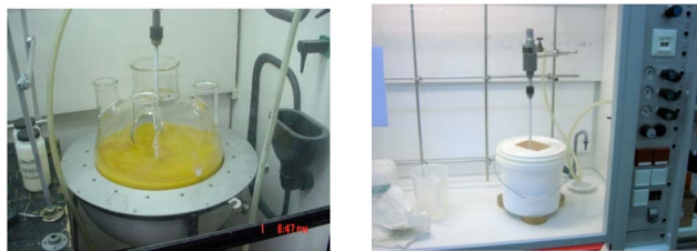
Fig. 1 High- and low-tech reactors for the synthesis of IPr·HCl.
