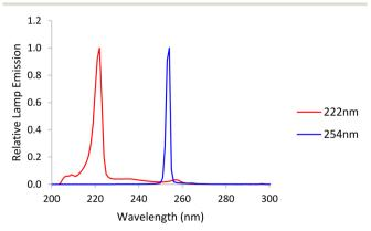
Fig. 1 Emission spectra from a low-pressure (LP) mercury lamp, labelled 254 nm, and a krypton-chloride excimer (KrCl\*) lamp, labelled 222 nm
