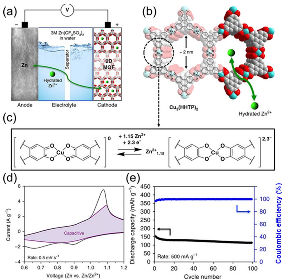
Fig. 10  $\text{Cu}_3(\text{HHTP})_2$  acting electrochemically as a cathode for rechargeable ZIBs. (a) Zn- $\text{Cu}_3(\text{HHTP})_2$  cell schematic depiction. (b) The  $\text{Cu}_3(\text{HHTP})_2$  chemical structure. (c) The anticipated redox mechanism in the  $\text{Cu}_3$  coordination unit (HHTP)<sub>2</sub>. (d) CV profile at  $0.5 \text{ mV s}^{-1}$ , together with the capacitive contribution (shaded region). (e) Cycling efficiency at  $500 \text{ mA g}^{-1}$ .<sup>157</sup>
