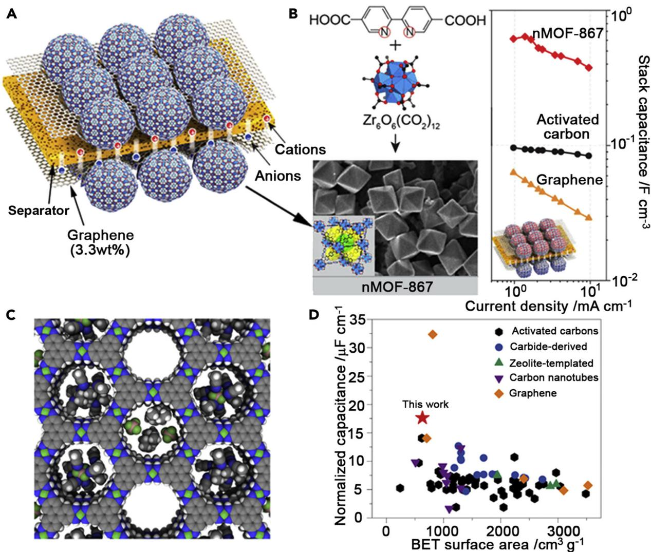
Fig. 3 MOF-based supercapacitors. (A) Schematic construction of MOF supercapacitors.<sup>53</sup> (B) Structure and nanocrystal morphology of nMOF-867 and comparison of stack capacitances among various EDLC materials.<sup>51</sup> (C) A space-filling diagram of idealized  $\text{Ni}_3(\text{HITP})_2$  (Ni, green; F, lime; N, blue; C, gray; B, brown; H, white).<sup>51</sup> (D) Comparison of BET-surface-area-normalized areal capacitances among various EDLC materials.<sup>54</sup>
