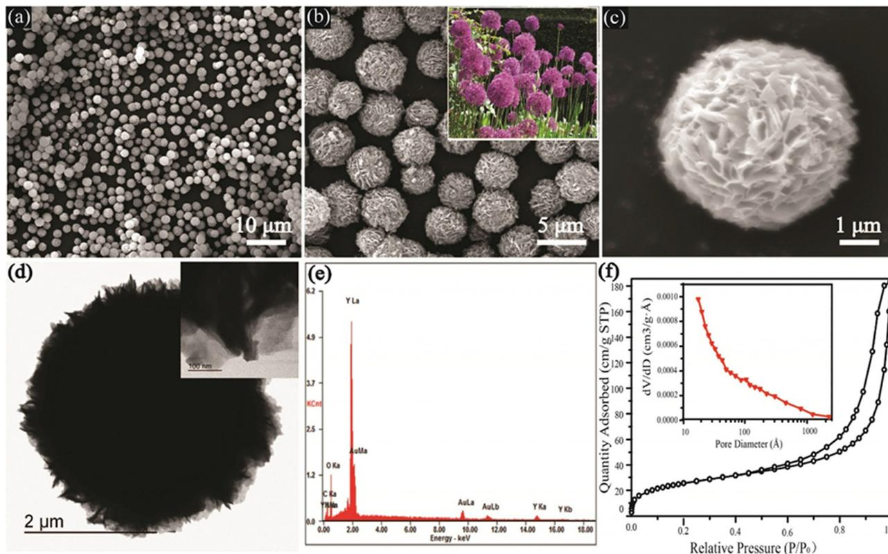
Fig. 1 SEM and TEM images of as-prepared Y-MOF samples at 120 °C for 24 h: (a)–(c) low- and high-magnification SEM images (inset in (b) is the photo of *Allium giganteum*);<sup>26</sup> (d) low- and high-magnification TEM images; (e) EDX spectrum;<sup>26</sup> (f) nitrogen adsorption/desorption isotherms of Y-MOFs:10%Eu<sup>3+</sup> (inset is pore size distribution).<sup>27</sup>
