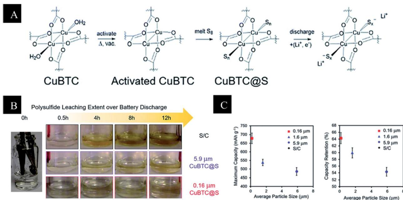
Fig. 7 (A) Activation and sulfur loading of HKUST-1 with potential binding sites at the Cu paddlewheel. (B) Electrolyte samples of 0.16  $\mu\text{m}$  and 5.9  $\mu\text{m}$  CuBTC, and S/C electrodes during a galvanostatic discharge of  $C/20$ . Yellow discoloration indicates the amount of leached polysulfide. (C) Coin cell performance of 3 cells as a function of particle size, left: the average maximum capacity and right: the average capacity retention over 20 cycles.<sup>117</sup>
