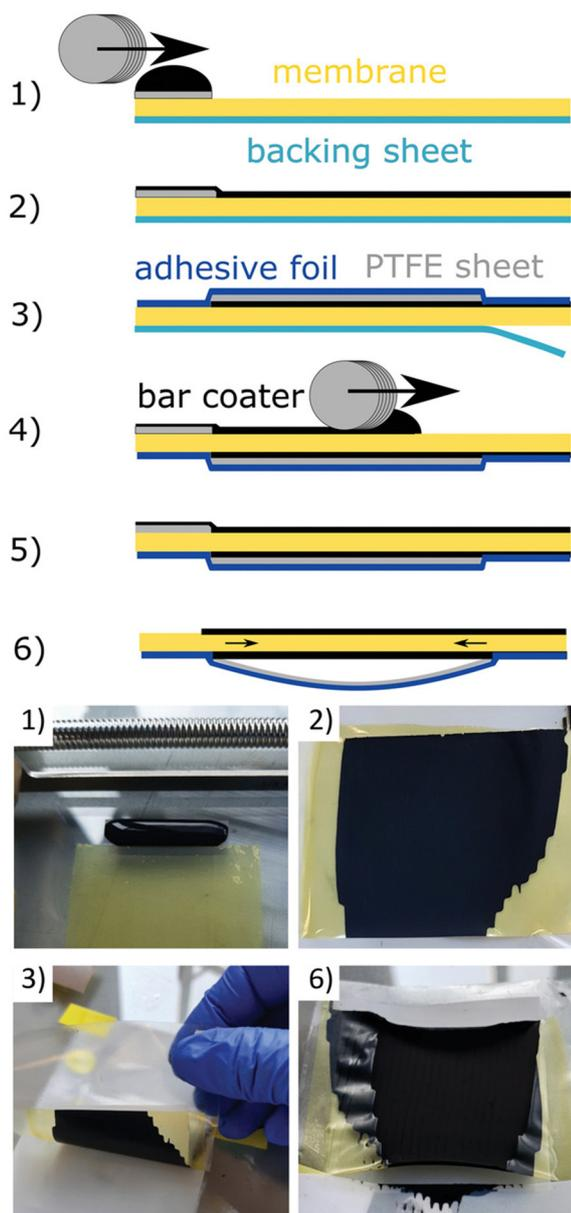
**Fig. 9** Fabrication steps of a directly coated CCM with bar coating method. (1), (2) use of the first catalyst layer; (3) use of a protective PTFE layer (grey) with an overlapping adhesive film (blue); (4), (5) use of the second catalyst layer Mayer-rod; (6) the PTFE layer creates gentle tension during drying/shrinking of the CL which protects the CCM from wrinkling. Reproduced with the permission from ref. 97. Copyright 2023, John Wiley and Sons.
