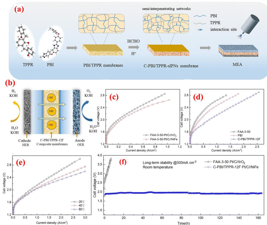
**Fig. 10** (a) preparation of PBI/TPPR and C-PBI/TPPR membrane; (b) constructed AEMWE system; (c) polarization curves of different anode catalysts in 1 M KOH at RT; (d) polarization curves of different membranes in 1 M KOH at RT; (e) polarization curves of C-PBI/TPPR-12F membrane at different temperatures; and (f) long-term stability test of commercial FAA-350 and C-PBI/TPPR-12F membranes at 500 mA cm<sup>-2</sup>. Reproduced with the permission from ref. 100. Copyright 2023, RSC.
