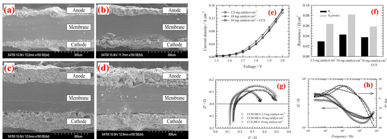
Fig. 7 Cross-sectional SEM pictures of the CCMs before (a), (c) and after (b), (d) AEMWE performance; (e) polarization curves of AEMWE with various membranes; (f) values of  $R_s$  and  $R_p$ ; (g) EIS; and (h) Bode plot. Reproduced with the permission from ref. 90. Copyright 2019, Elsevier.
