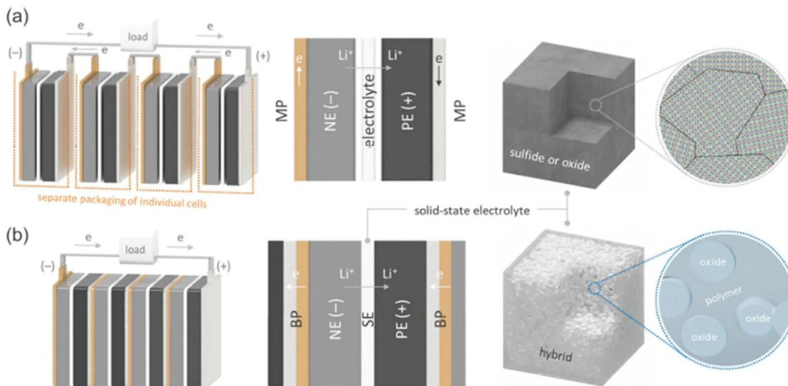
Fig. 10 Schematic diagrams of (a) the monopolar design of current LIBs with liquid electrolytes and (b) bipolar design of SSLBs equipped with SEs. The  $\text{Li}^+$  and electron pathways during discharge are also indicated. (Reproduced with permission from ref. 63).
