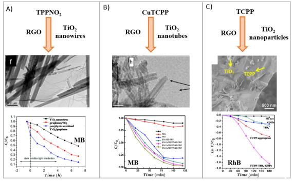
Fig. 30 Ternary nanostructures of various porphyrin/RGO/TiO2 composites and their photocatalytic performance. Adapted with permission from ref. 149, 151 and 153. Copyright 2014 Elsevier B.V, 2016 Hydrogen Energy Publications LLC, 2015 Elsevier Inc.
