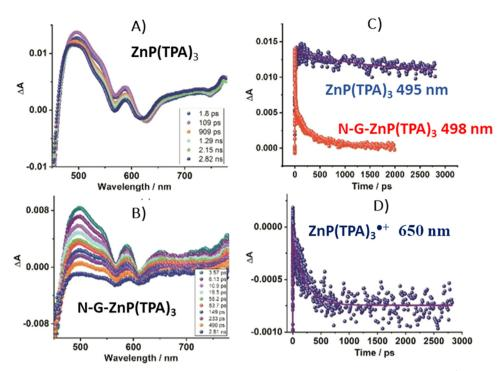
Fig. 20 Femtosecond TAS at indicated delay times for (A) ZnP(TPA)<sub>3</sub> control and (B) its hybrid with N-G, (C) TA decays for <sup>1</sup>ZnP(TPA)<sub>3</sub>\*: control at 495 nm (free porphyrin) and hybrid at 498 nm (porphyrin bound to N-G), (D) time profile for the 650 nm peak corresponding to ZnP(TPA)<sub>3</sub>\*\*. Adapted from ref. 113.
