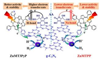
Fig. 35 ZnMT3PyP and ZnMTPP sensitized graphitic carbon nitride for efficient visible light-driven H2 production. Reproduced form ref. 161. Copyright 2017, American Chemical Society.
