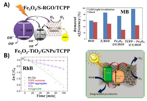
Fig. 33 (A) Mechanism of MB photodegradation catalyzed by Fe<sub>3</sub>O<sub>4</sub>/S-RGO/TCPP. Adapted with permission from ref. 156. Copyright 2015, Springer Science Business Media Dordrecht. (B) Mechanism of RhB photodegradation catalyzed by Fe<sub>2</sub>O<sub>3</sub>-TiO<sub>2</sub>/GNPs/TCPP. Adapted with permission from ref. 155. Copyright 2021 Elsevier Ltd
