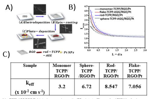
Fig. 22 (A) Scheme of the TCPP-AGG/RGO/Pt fabrication procedure on the ITO substrate, (B) normalized SECM feedback curves recorded for different TCPP-AGG/RGO/Pt films on ITO, and (C) morphology-dependent apparent/effective PET rate constants (kerf) for samples with various porphyrin aggregates, obtained from simulating the experimental SECM curves presented in B. Adapted with permission from ref. 119. Copyright 2018 Elsevier Ltd.
