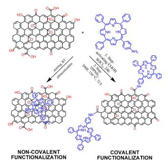
Fig. 1 Schematic of the process of preparation of GO with covalently (Por-GO) and non-covalently (Por/GO) linked porphyrins. The conditions for covalent functionalization were taken from ref. 58.
