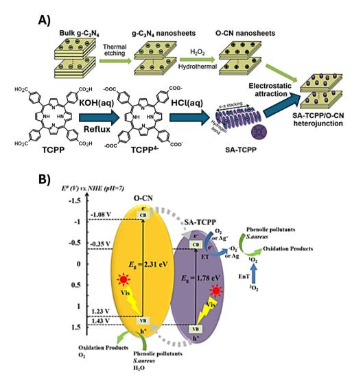
Fig. 39 (A) Synthesis of g-C<sub>x</sub>N<sub>4</sub>-O, SA-TCPP and SA-TCPP/g-C<sub>x</sub>N<sub>4</sub>-O heterojunctions and (B) schematic representation of the proposed carrier separation and photocatalytic processes under visible light irradiation in the SA-TCPP/q-C<sub>3</sub>N<sub>4</sub>-O heterojunction catalyst. Reproduced from ref. 168 Copyright 2021 Elsevier.
