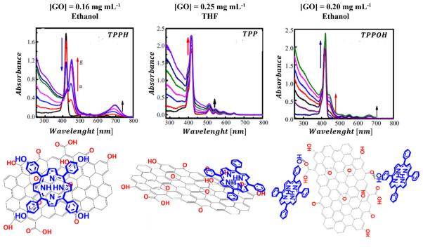
UV-vis absorption spectra and structural schemes of TPPH/GO, TPP/GO, and TPPOH/GO. Adapted with permission from ref. 95. Copyright 2015 Elsevier.
