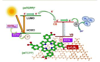
Fig. 37 Mechanism of photocatalytic hydrogen production from water over g-C<sub>3</sub>N<sub>4</sub> sensitized with m-TCPP porphyrin. Reproduced from ref. 163. Copyright 2018 Elsevier.
