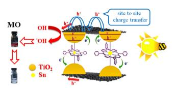
Fig. 32 Diagram depicting the charge transfer process in the prepared SnTCPP/graphene/TiO<sub>2</sub> hybrid exposed to visible light irradiation. Adapted with permission from ref. 152. Copyright © 2015 Elsevier Inc.
