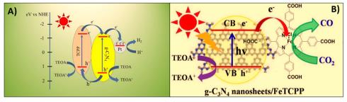
Fig. 36 (A) Suggested mechanism for photocatalytic  $H_2$  evolution over TCPP/g- $C_3N_4$ /Pt under visible light irradiation ( $\lambda > 380$  nm). Reproduced from ref. 162. Copyright 2017 Elsevier. (B) Structure of the g-C<sub>3</sub>N<sub>4</sub>/FeTCPP heterogeneous catalyst. Adapted from ref. 171, Copyright 2018 Elsevier.
