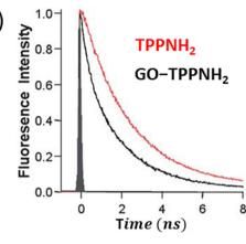
Fig. 15 Comparison of the (A) fluorescence spectra and (B) fluorescence decay profiles of free porphyrin TPPNH<sub>2</sub> versus the porphyrin covalently bound to GO. Adapted with permission from ref. 59. Copyright 2011, Royal Society of Chemistry.
