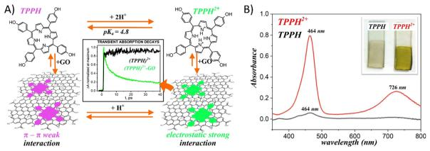
Fig. 9 (A) Schematic of the pH influence on the interaction of TPPH with GO. (B) Comparison of the adsorption of porphyrins (TPPH (black) and cationic TPPH<sup>2+</sup> (red)) from solutions on GO films monitored by UV-vis spectroscopy. Adapted with permission from ref. 72. Copyright 2019 American Chemical Society.
