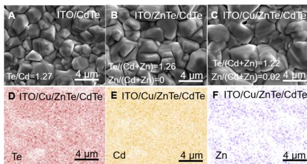
Fig. 2 Plan-view SEM image (A–C) and SEM-EDS mapping results for ITO/Cu/ZnTe/CdTe (D–F). Composition ratios of Te/(Cd + Zn) and Zn/(Cd + Zn) obtained by simultaneously performed SEM-EDS analysis are expressed in the SEM images.
