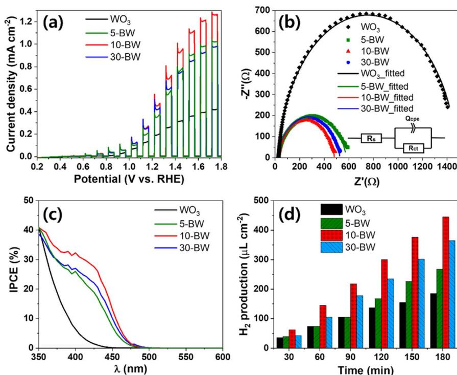
Fig. 4 Photoelectrochemical performances of the  $\text{WO}_3$  nanocrystals and  $\text{BiVO}_4/\text{WO}_3$  photoanodes of 5-BW, 10-BW, and 30-BW: (a) photocurrent densities by linear sweep voltammetry, (b) Nyquist plots and equivalent circuits, (c) PEC  $\text{H}_2$  production diagram as a function of time, and (d) IPCE spectra.
