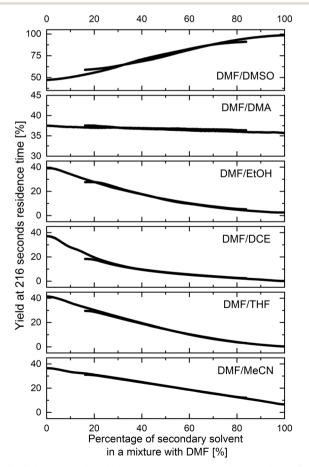
Fig. 3 Selected results of binary solvents mixtures flow studies in S<sub>N</sub>Ar reaction.
