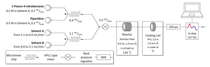
Fig. 2 Flow setup and reaction conditions used in solvents mixtures studies in S<sub>N</sub>Ar reaction.
