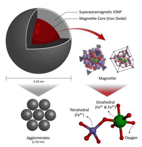
Fig. 6 (a) Superparamagnetic iron oxide nanoparticles (SPIONs). (b) Face-centered cubic (FCC) closed packing, with  $Fe^{3+}$  in the tetrahedral sites and  $Fe^{2+}$  occupying the octahedral sites.
