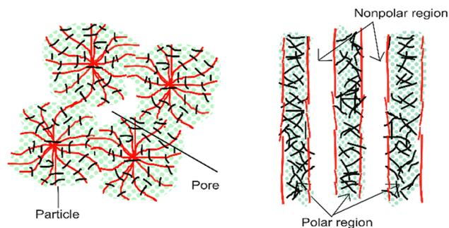
Fig. 6 Illustration of the polarity distribution between disordered (left) and more oriented nanofibers (right).<sup>15</sup>
