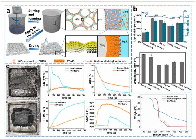
Fig. 5 (a) Preparation process of foam finishing; (b) liquid carrying rate and air permeability of fabric treated by different means, <sup>127</sup> Copyright 2021 Elsevier; (c) fabric cone calorimetry and thermogravimetric test, <sup>128</sup> Copyright 2023 Elsevier.
