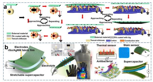
Fig. 11 (a) Structure and working principle of friction nanogenerator, <sup>187</sup> Copyright 2021 American Chemical Society; (b) wearable supercapacitors and human motion sensors, 191 Copyright 2021 American Chemical Society.
