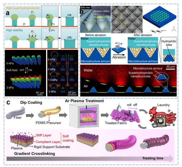
Fig. 7 (a) Design of the LPGSS and its switching effect diagram, <sup>132</sup> Copyright 2022 Wiley-VCH; (b) design of the microstructure armour, <sup>133</sup> Copyright 2020 Springer Nature; (c) SH fabric is prepared by argon plasma treatment and a wrinkled surface is formed on the fiber, 134 Copyright 2021 American Chemical Society.
