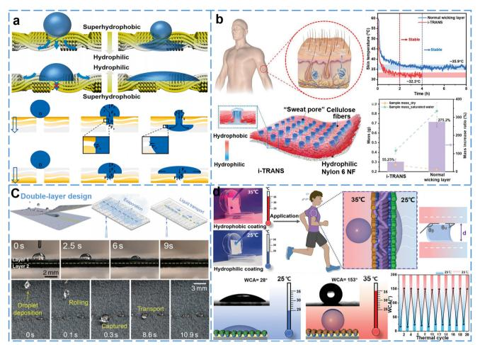
Fig. 9 (a) Janus fabric one-way water transport mechanism, 127 Copyright 2021 Elsevier; (b) concept illustration of integrated 3D hydrophilicity/ hydrophobicity design for artificial sweating skin (i-TRANS), <sup>169</sup> Copyright 2022 Wiley-VCH; (c) schematic of the fabrication of the double-layer fabric assembly, <sup>170</sup> Copyright 2023 The Royal Society of Chemistry; (d) temperature triggered directional water transport fabric, <sup>171</sup> Copyright 2023 Wiley-VCH.
