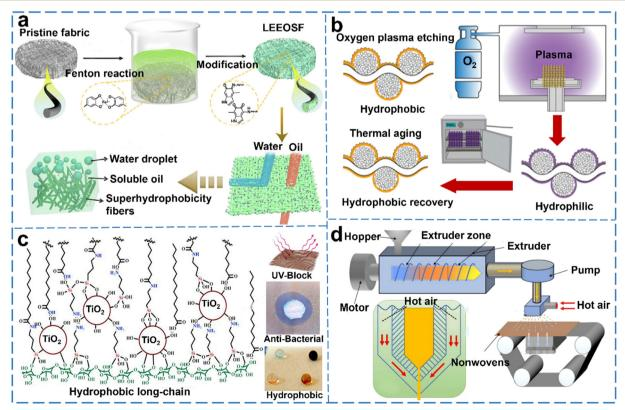
Fig. 4 Preparation of superhydrophobic fabric by (a) Fenton reaction,<sup>116</sup> Copyright 2023 Elsevier; (b) oxygen plasma etching and thermal aging,<sup>117</sup> Copyright 2020 Elsevier; (c) hydrophobic branches on fabric long chains,<sup>118</sup> Copyright 2023 Elsevier; (d) melt-blow method,<sup>119</sup> Copyright 2022 MDPI.
