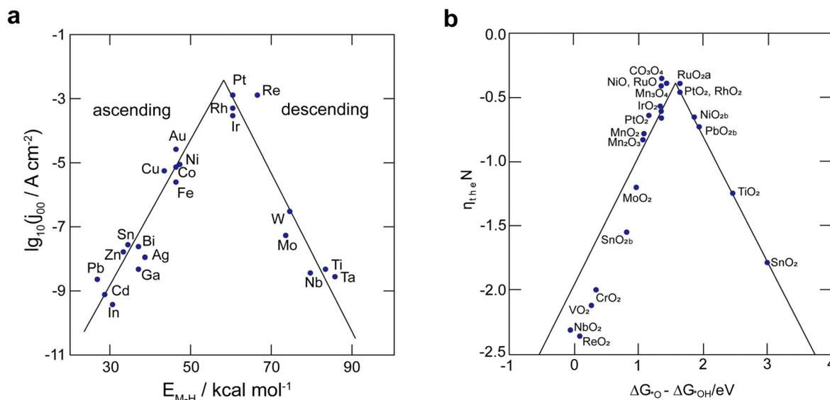
Fig. 5 (a) Catalyst activity for the HER in an acidic solution presented as a volcano plot, depicting the connection between hydride formation energy ( $E_{M-H}$ ) and current density ( $j_{00}$ ). (b) Volcano plot showcasing the activity of catalysts for OER, displaying overpotential in relation to the standard free energies of various metal oxides.
