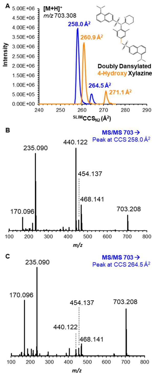
Fig. 3 (A) Ion mobilogram for 3-hydroxy and 4-hydroxy xylazine as the protonated doubly dansylated products at  $m/z$  703. Each individual mobility peak, at (B) CCS 258.0 and (C) CCS 264.5 Å<sup>2</sup>, was subjected to mobility-aligned fragmentation (MAF), for which their spectra are shown above.
