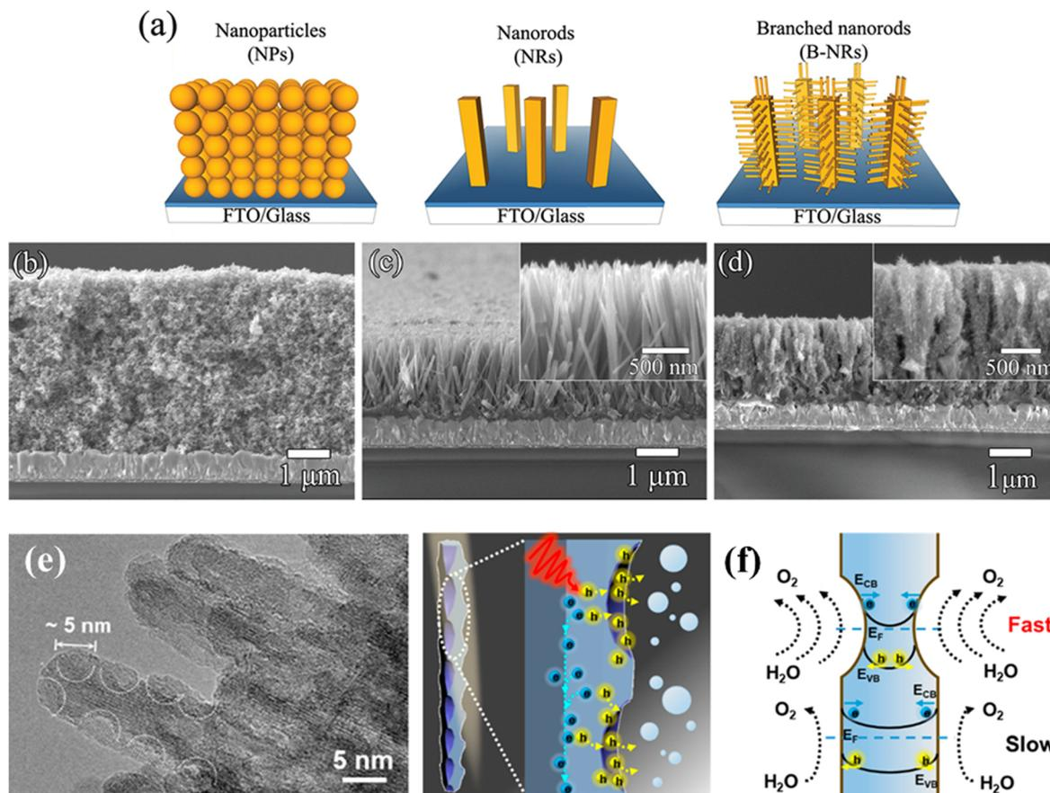
**Fig. 5** (a) Schematic diagram of the synthesis of TiO<sub>2</sub> branched nanorods. SEM images of (b) TiO<sub>2</sub> nanoparticles, (c) nanorods, and (d) branched nanorods. Reprinted with permission from ref. 43. Copyright © 2011, American Chemical Society. (e) TEM image of the TiO<sub>2</sub> nanowire arrays. (f) Schematic illustrations of the hole extraction effect of TiO<sub>2</sub> nanowire arrays. Reprinted with permission from ref. 45. Copyright © 2022, American Chemical Society.
