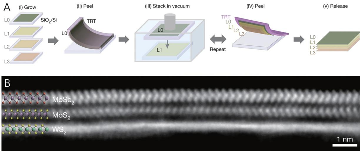
**Fig. 3** (A) A schematic of the programmed vacuum stack (PVS) process. (B) The cross-sectional STEM image of a MoSe<sub>2</sub>/MoS<sub>2</sub>/WS<sub>2</sub> film with the electron beam aligned with the armchair axis of MoSe<sub>2</sub> (top) and MoS<sub>2</sub> (middle). Reproduced with permission from ref. 59, copyright Springer Nature.
