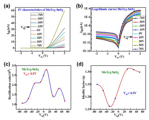
Fig. 4 (a)  $I_{ds}$  –  $V_{ds}$  characteristic curves of the MoTe<sub>2</sub>–SnS<sub>2</sub> heterostructure at various back gate voltages ( $V_{bq}$ ); the linear scale. (b) Logarithmic scale. The maximum rectification ratio is  $2.79 \times 10^5$  mA W<sup>-1</sup>. (c) The change in the rectification ratio of the device at various back gate voltages. (d) The variation in the ideality factor at different gate voltages.
