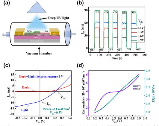
Fig. 6 (a) Schematic of the p-n device for photodetection. (b) Photocurrent at  $V_q = 0$ , for  $V_{ds} = 0.2 - 0.9$  V with incident light ( $\lambda = 220$  nm) and power intensity 11 mA cm<sup>-2</sup>. (c) I-V curves in the dark and under light, representing  $I_{SC} = -8.5$  nA and  $V_{OC} = 0.20$  V at  $V_{q} = 0$ . (d) The change in responsivity at different values of  $V_{\rm ds}$ . (e) The enhancement in the EQE at different values of  $V_{\rm ds}$ .
