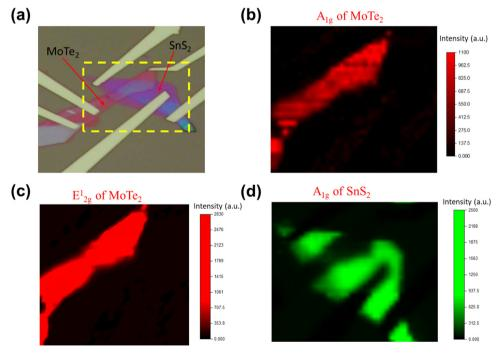
Fig. 2 (a) Optical image of the device that shows the area selected for Raman mapping. (b) Raman intensity maps of  $A_{1g}$  of MoTe<sub>2</sub>. (c) Raman intensity maps of  $E_{2g}^1$  of MoTe<sub>2</sub>. (d) Raman intensity maps of  $A_{1g}$  of SnS<sub>2</sub>. Graphical representation of Raman intensity mapping at 172.43 and 232.93 cm<sup>-1</sup> for MoTe<sub>2</sub>, and  $315.78~\text{cm}^{-1}$  for SnS<sub>2</sub>.
