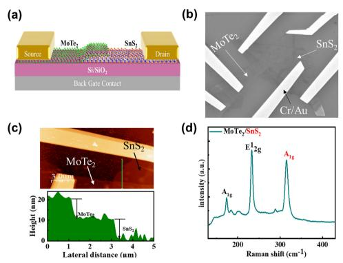
Fig. 1 (a) Schematic illustration of the p-n device. (b) SEM image of the p-n heterostructure  $MoTe_2-SnS_2$ -based device; the scale bar is 5  $\mu$ m. (c) AFM profile of the heterostructure. (d) Raman spectra of the MoTe<sub>2</sub>-SnS<sub>2</sub> heterostructure.
