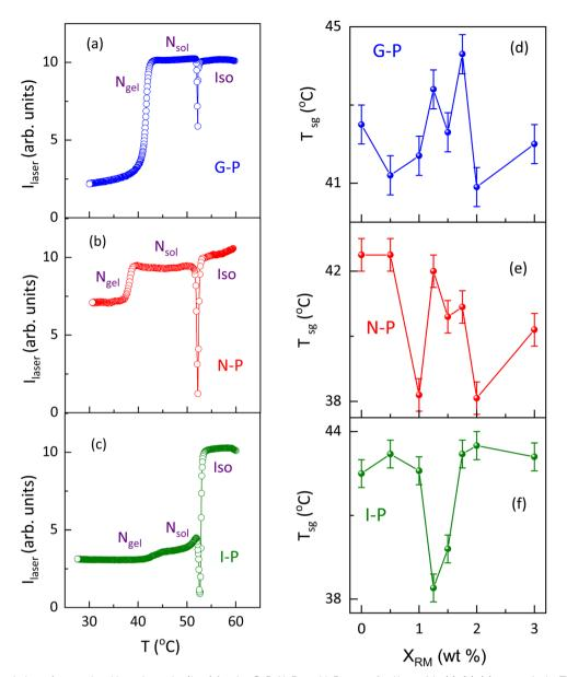
Fig. 10 Thermal variation of transmitted laser intensity (I<sub>laser</sub>) for the G-P, N-P, and I-P cases, for X<sub>RM</sub> = 1 in (a), (b), (c) respectively. The variation of T<sub>sq</sub> with different  $X_{\rm RM}$  is shown for the G-P, N-P, and I-P cases in (d), (e), (f), respectively.
