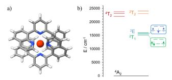
Fig. 4 (a) DFT optimized geometry of the quartet ground state of [Cr(dqp)<sub>2</sub>]<sup>3+</sup>. Spin density at the Cr center: 3.151647. (b) Schematic representation of the energy levels for the calculated (CASSCF(7,12)-FIC-NEVPT2) excited states of [Cr(dqp)<sub>2</sub>]<sup>3+</sup>
