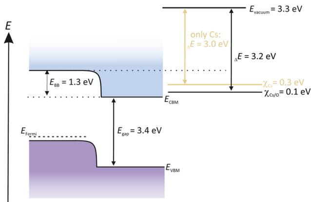
Fig. 12 Schematic representation of the band structure of p-GaN when activated with Cs and O<sub>2</sub>.
