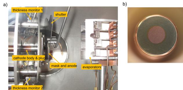
Fig. 6 (a) The interior of the Cs<sub>2</sub>Te preparation chamber, showing a cathode body with a plug, shutter, a mask which is also an anode, two thickness monitors, and Cs and Te evaporators and (b) photo of a freshly deposited Cs<sub>2</sub>Te layer (4 mm in diameter) on a Cu plug.
