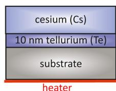
Fig. 5 Schematic overview of a typical layer sequence for a Cs<sub>2</sub>Te photocathode, based on the original approach taken from ref. 40.
