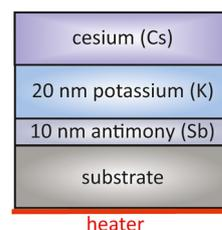
Fig. 7 Schematic overview of a typical layer sequence for a K<sub>2</sub>CsSb photocathode, based on the original approach taken from ref. 51.
