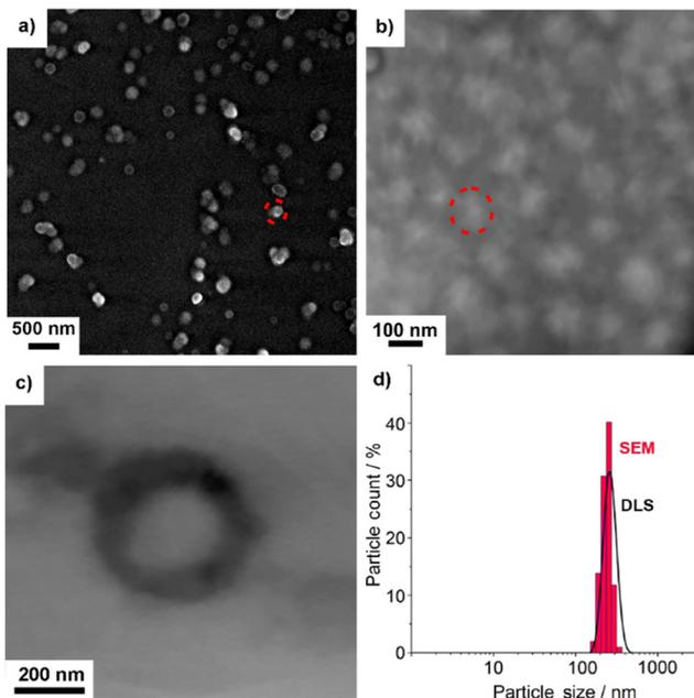
Fig. 2 Size and structure of the as-prepared AMC@SiO<sub>2</sub> core@shell nanocarriers: (a and b) SEM overview images at different levels of magnification with selected nanocarriers indicated by red dots, (c) STEM detail image, (d) size distribution according to SEM and DLS.
