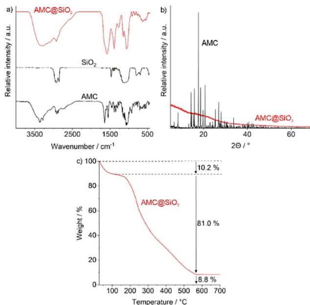
Fig. 4 Chemical composition of the as-prepared AMC@SiO<sub>2</sub> core@shell nanocarriers: (a) FT-IR spectrum with pure AMC and SiO<sub>2</sub> as references, (b) XRD with AMC as a reference, (c) TG analysis.
