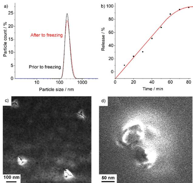
Fig. 6 AMC release of AMC@SiO<sub>2</sub> core@shell nanocarriers: (a) particle size according to DLS analysis prior and after freezing in DMSO at  $-30\text{ }^{\circ}\text{C}$  for 10 weeks, (b) UV-vis spectra showing the AMC release after mixing of DMSO suspensions with water based on the NFR absorption (at 535 nm) in the supernatant after 10–80 min of stirring and separation of the nanocarriers, (c) and (d) SEM images of nanocarriers after AMC release with considerable cracks in the surface.
