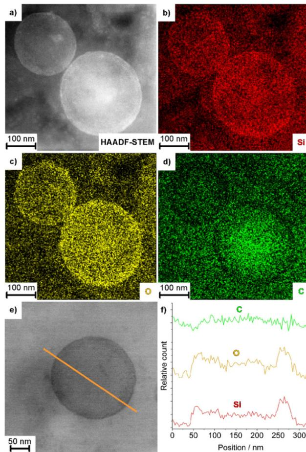
Fig. 3 Nanostructure of AMC@SiO<sub>2</sub> core@shell nanocarriers: (a) HAADF-TEM image, (b–d) EDXS area scans (Si–K, O–K, C–K lines used for analysis) of the nanostructure shown in (a), (e and f) EDXS line scan with (f) element mapping along the orange line in (e).
