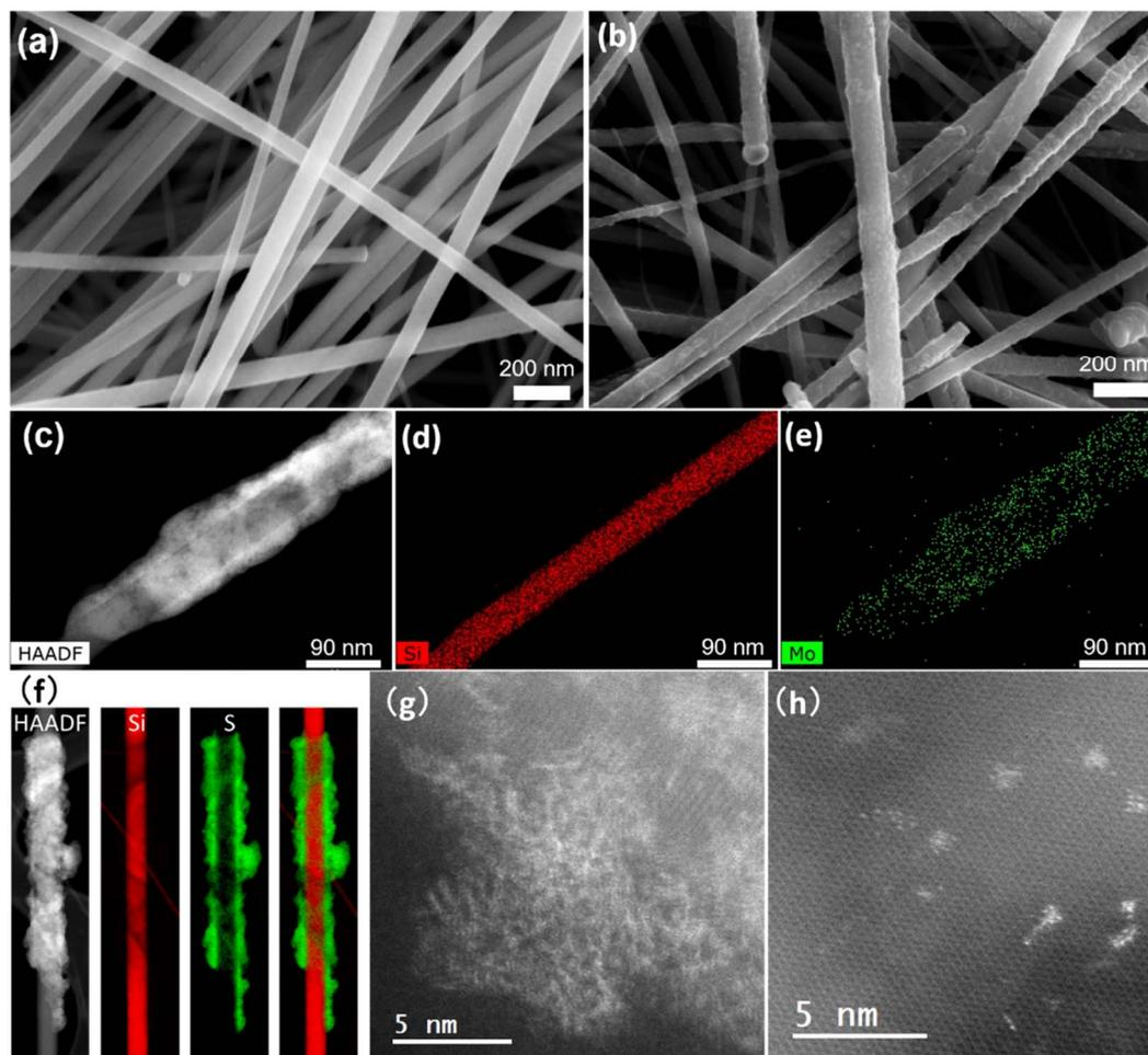
Fig. 4 SEM images of (a) 48 nm-SiNWs, (b) SiNW-MoS<sub>x</sub> with  $\Delta Q = 6 \text{ mC cm}^{-2}$  (c) HAADF-STEM image of SiNW-MoS<sub>x</sub> and EDX mapping profile of (d) Si(K<sub>α</sub>) and (e) Mo(K<sub>α</sub>); (f) STEM-HAADF image and EELS mapping profile of element Si (L edge at 99 eV) and S (L edge at 165 eV); (g, h) High-resolution HAADF-STEM images of a-MoS<sub>x</sub>.
