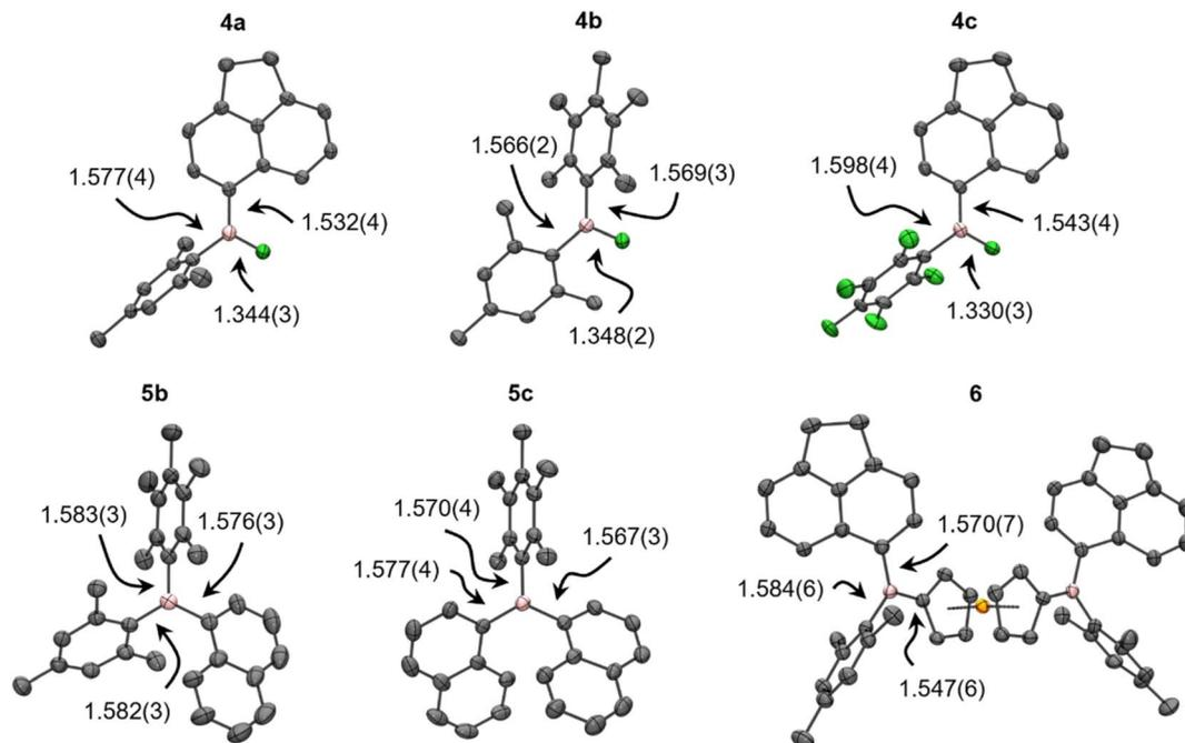
Fig. 2 Thermal ellipsoid plots of diaryl- (**4**, 150 K, 50% probability level) and triarylboranes (**5b**, **5c** and **6**, 298 K, 20% probability level), with B–C and B–F bond lengths (in Å). Colours denote Fe (orange), F (green), B (pink), and C (grey), with H atoms omitted for clarity.
