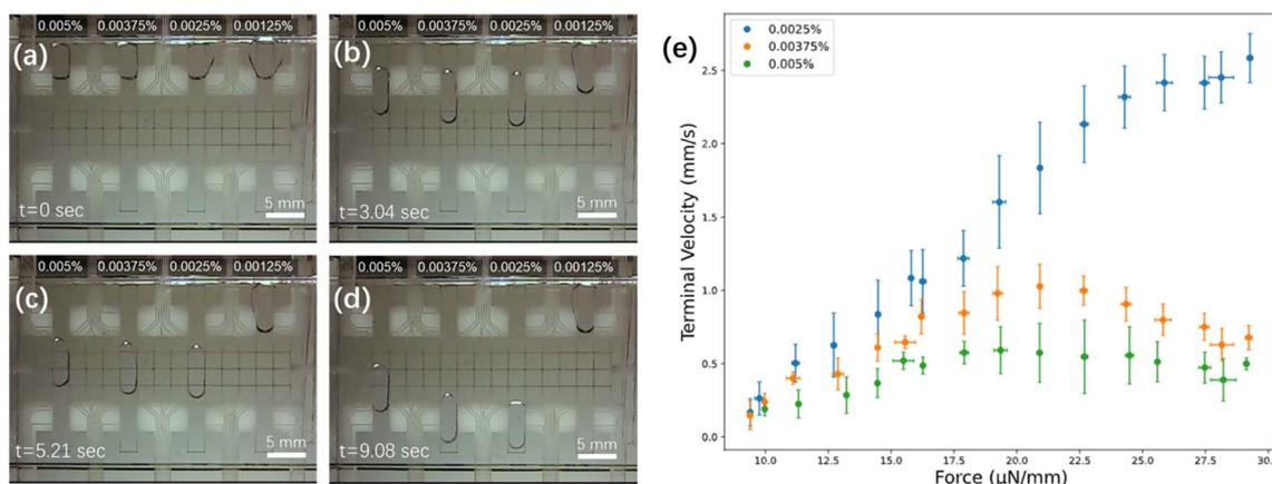
Fig. 2 Effect of DDM concentration on droplet movement. Frames from Movie S1<sup>†</sup> illustrating the movement of aqueous droplets containing DDM (0.0025, 0.00375, and 0.005% wt/wt) after (a) 0 s (during the loading step), (b) 3.04 s, (c) 5.21 s, and (d) 9.08 s. (e) Force–velocity curves for the three highest concentrations tested (0.0025% – blue, 0.00375% – orange, 0.005% – green). Error bars are  $\pm 1$  st. dev. for  $n = 3$  replicates per condition.
