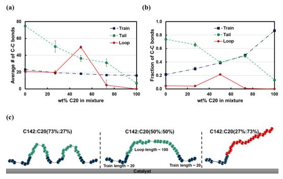
Fig. 7 Effects of  $C_{20}$  concentration in binary mixtures of  $C_{20}$  and  $C_{142}$  over Pt(111) at 473 K on (a) the average length of trains, tails and loops of both  $C_{20}$  and  $C_{142}$  in the mixture combined, and (b) the fraction of C-C bonds belonging to trains, tails and loops. (c) Cartoons of representative conformations of the  $C_{142}$  chain on Pt(111) for  $C_{142}$ :  $C_{20}$  mixtures of varying  $C_{20}$  concentrations. Error bars represent one standard deviation.
