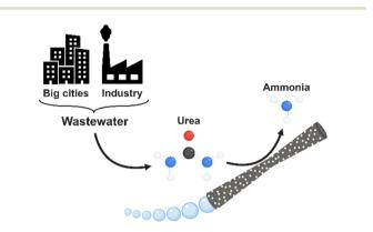
Fig. 1 Ammonia generation and pollutant removal by MnO<sub>2</sub>-based tubular micromotors.
