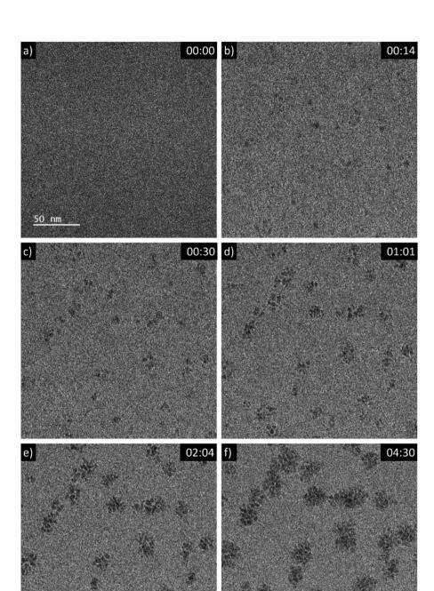
Fig. 1 Sequential images from an *in situ* LP-TEM movie showing the formation of aggregates (see video "V01\_LP-TEM\_CeO<sub>2</sub>-nanoparticles.avi", time given as mm:ss). A dose rate of  $16.7 \times 10^6$  Gy s<sup>-1</sup> is applied.
