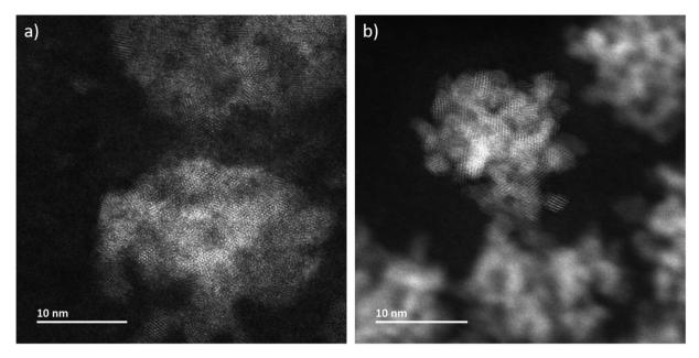
Fig. 3 ADF-STEM images of  $CeO_2$  grown (a) in LP-TEM (dose rate 16.7  $\times$  10<sup>6</sup> Gy s<sup>-1</sup>) and (b) under steady-state gamma radiolysis.
