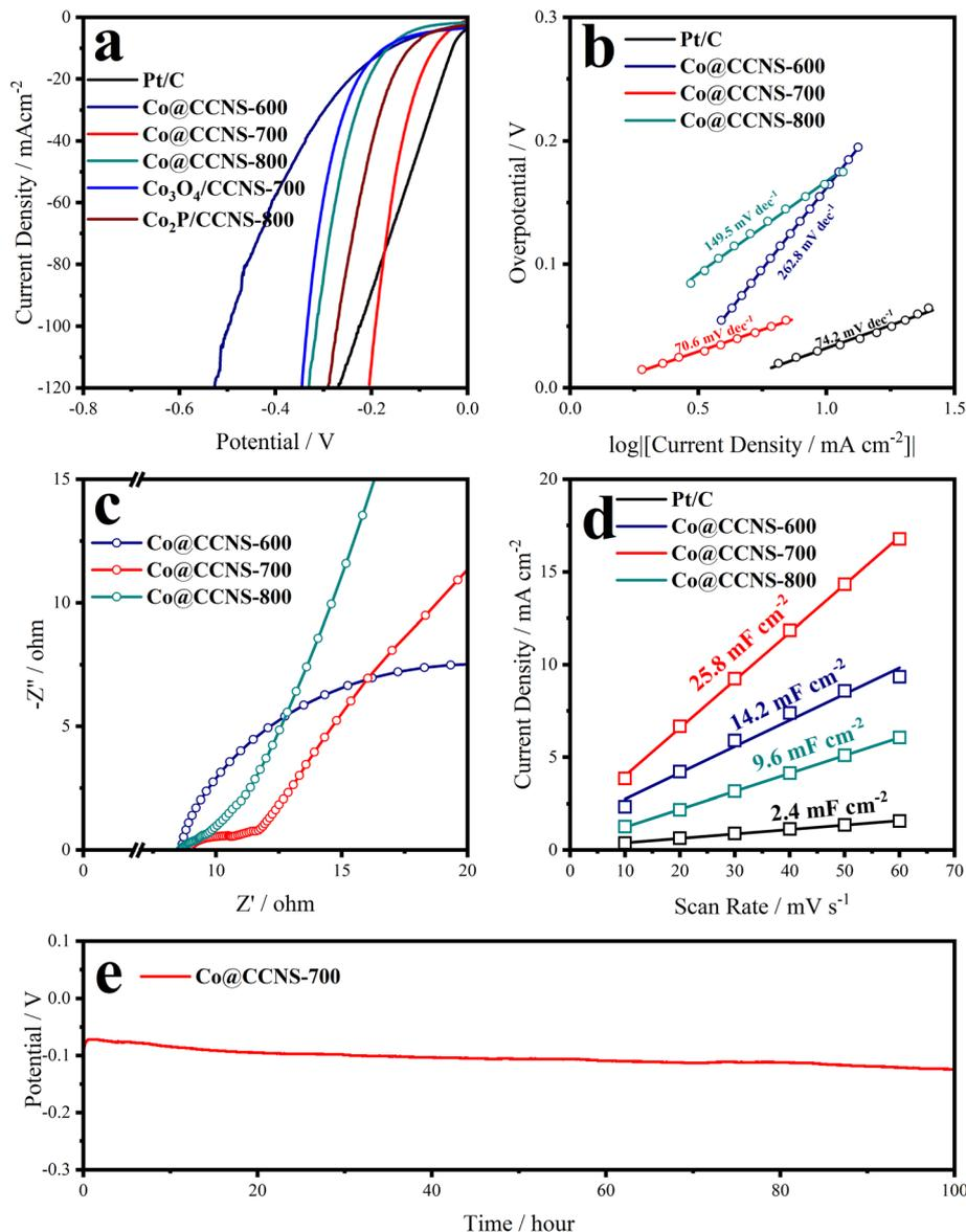
**Fig. 4** (a) 95%  $iR$ -corrected linear sweep voltammetry (LSV), (b) Tafel slopes, (c) electrochemical impedance spectroscopy, and (d) the electric double layer capacitances from current-scan rate relationships at 1.0 V (vs. RHE) plots of Co@CCNSs. (e) Electrochemical stability test of Co@CCNS-700 under a fixed current density of  $10 \text{ mA cm}^{-2}$ .
