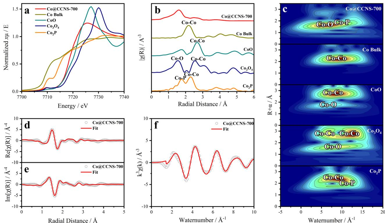
**Fig. 5** (a) Normalized X-ray absorption near edge structure (XANES) spectra of cobalt k-edge in  $\text{Co@CCNS-700}$ . (b) Fourier transform and (c) wavelet transform on extended X-ray absorption fine structure (EXAFS) data of  $\text{Co@CCNS-700}$ . Fittings of (d) real part and (e) imaginary part of *R*-space and (f) *k*-space EXAFS plots of  $\text{Co@CCNS-700}$ .
