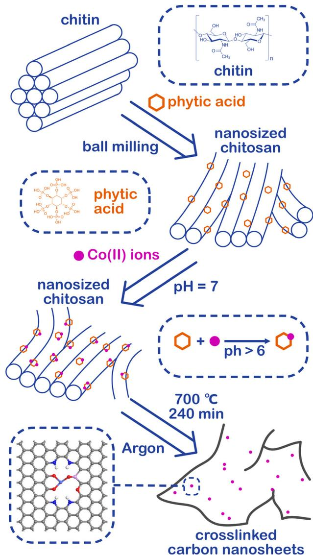
Fig. 1 Preparation flow chart of cobalt SACs loaded crosslinked carbon nanosheets (Co@CCNS).
