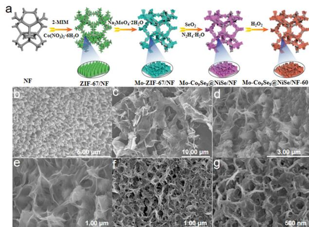
**Fig. 1** (a) Schematic illustration of the preparation of Mo-Co<sub>9</sub>Se<sub>8</sub>@NiSe/NF-60. SEM images of (b) ZIF-67/NF, (c) Mo-ZIF-67/NF, (d and e) Mo-Co<sub>9</sub>Se<sub>8</sub>@NiSe/NF, and (f and g) Mo-Co<sub>9</sub>Se<sub>8</sub>@NiSe/NF-60.
