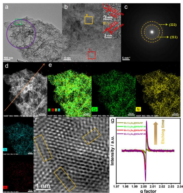
**Fig. 2** (a) TEM image, (b) HRTEM images (inset I-1 and II-2 correspond to the area of red square I and orange square II), (c) SAED patterns, (d) HAADF-STEM images, (e) EDX images, and (f) local HRTEM images of Mo-Co<sub>9</sub>Se<sub>8</sub>@NiSe/NF-60. (g) EPR spectra of etched Mo-Co<sub>9</sub>Se<sub>8</sub>@NiSe/NF with different etching durations compared to Mo-Co<sub>9</sub>Se<sub>8</sub>@NiSe/NF.
