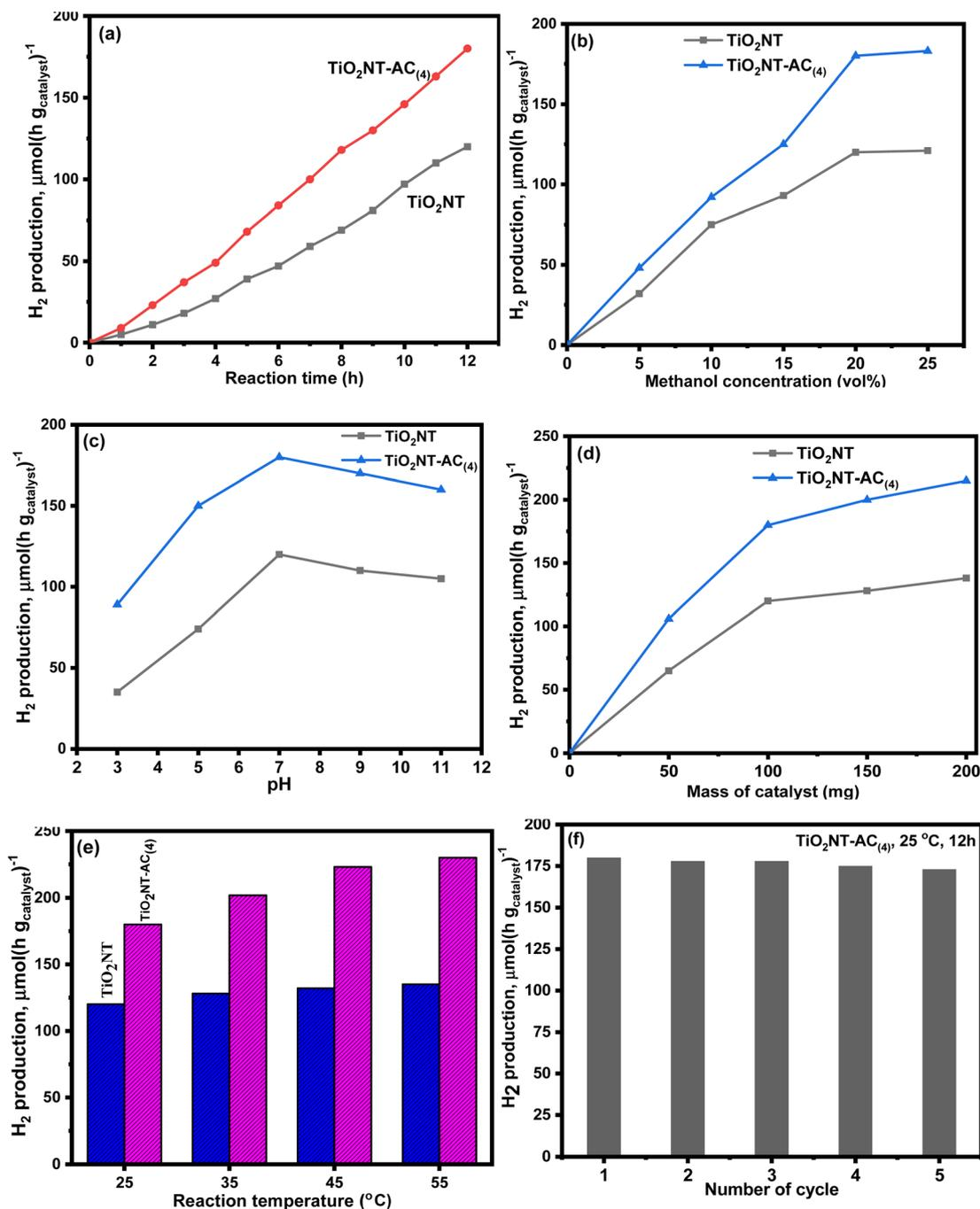
Fig. 9 Photocatalytic hydrogen production over synthesized  $\text{TiO}_2\text{NTs}$  and  $\text{TiO}_2\text{NTs-AC}_{(4)}$  catalysts. (a) effect of reaction time, (b) effect of concentration of methanol, (c) effect of solution pH, (d) effect of mass of catalysts, (e) effect of reaction temperature, and (f) recyclability of the  $\text{TiO}_2\text{NTs-AC}_{(4)}$  catalyst.
