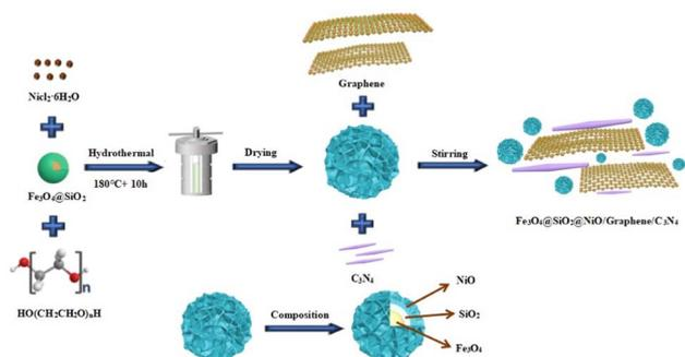
Fig. 1 Formation of the  $\text{Fe}_3\text{O}_4@SiO_2@NiO$  (FSN)/graphene/ $C_3N_4$  composites.
