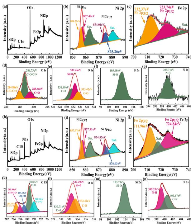
Fig. 4 XPS spectra of the Fe<sub>3</sub>O<sub>4</sub>@SiO<sub>2</sub>@NiO magnetic nanoparticles (FSN MNPs): (a) survey, (b) Ni 2p, (c) Fe 2p, (d) C 1s, (e) O 1s, (f) Si 2s, and (g) N 1s. XPS spectra of the FSN/Gr/C<sub>3</sub>N<sub>4</sub> composites: (h) survey, (i) Ni 2p, (j) Fe 2p, (k) C 1s, (l) O 1s, (m) Si 2s, and (n) N 1s.
