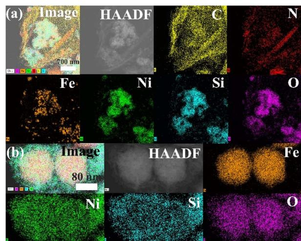
Fig. 3 STEM-HAADF and elemental mapping images of (a)  $Fe_3O_4@SiO_2@NiO$  (FSN)/Gr/ $C_3N_4$  and (b) FSN magnetic nanoparticles (MNP)—elemental Fe (brown), Ni (green), Si (cyan), O (pink), C (yellow), and N (red) mapping.
