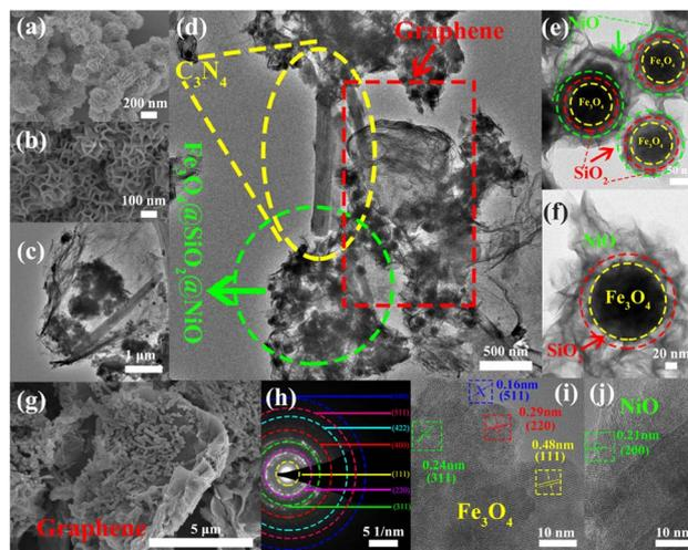
Fig. 2 (a and b) SEM images of the  $Fe_3O_4@SiO_2@NiO$  magnetic nanoparticles (FSN MNPs); TEM images of (c and d) FSN/Gr/ $C_3N_4$  and (e and f) FSN MNPs; (g) SEM image of FSN/Gr/ $C_3N_4$ ; (h) SAED image of the  $Fe_3O_4$  MNPs; (i) HRTEM images of  $Fe_3O_4$ ; (j) HRTEM images of NiO.
