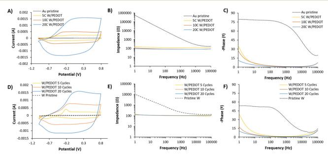
Fig. 4 (A) Cyclic voltammetry, impedance (B) and (C) phase measured of bare tungsten (W) and 5, 10 and 20 cycles coated W/PEDOT in 0.1× PBS as supporting electrolyte in water, (D) cyclic voltammetry, impedance (E) and (F) phase measured of bare gold (Au) and 5, 10 and 20 cycles coated Au/PEDOT in same conditions.
