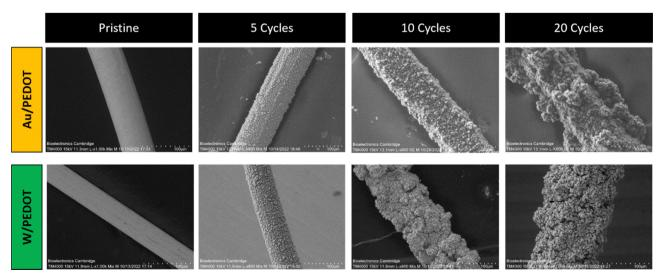
Fig. 3 SEM of pristine Au and W microwires and Au/PEDOT and W/PEDOT electropolymerized at 5, 10 and 20 cycles in 10 mL of ACN, 0.1 M EDOT and 0.1 M of TBAClO<sub>4</sub> (scale bar: 100  $\mu$ m).
