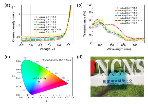
Fig. 5 (a) J-V curves of PBDTTPTP:N3 semitransparent solar cells with different D/A ratios. (b) Transmittance spectra. (c) Coordinates of CIE 1931 for the best-LUE cell. (d) The photograph of a 1 cm<sup>2</sup> semitrasparent cell made under optimal conditions.
