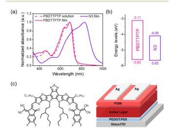
Fig. 3 (a) Absorption spectra of PBDTTPTP in solution and film states and N3 film. (b) Energy level diagram. (c) The chemical structure of N3 and the conventional device structure.
