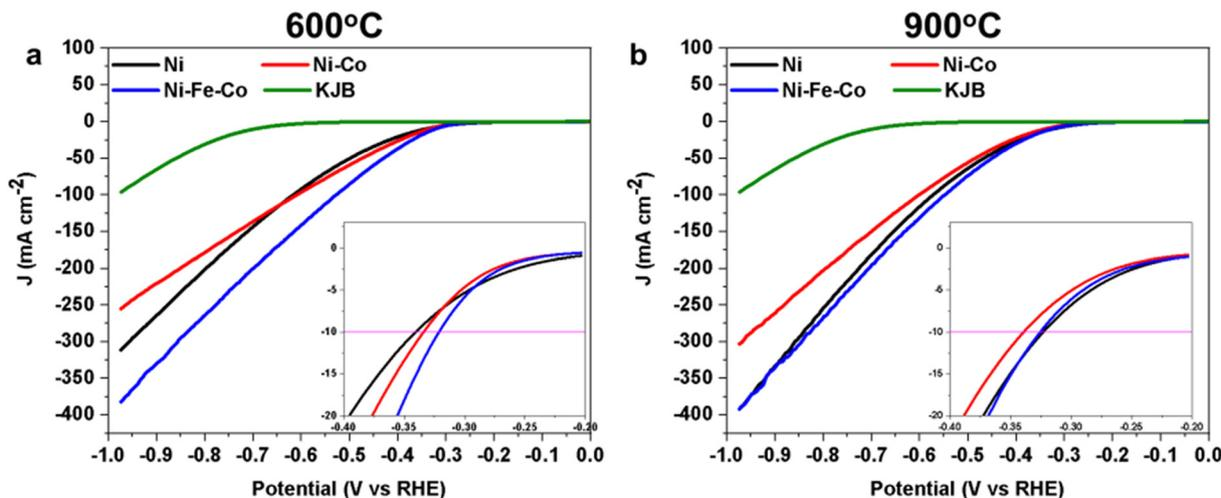
**Fig. 11** The LSVs of RDE measurement for the KJB Ni-based electrocatalysts with different compositions of materials and different thermal treatment temperatures of (a) 600 °C and (b) 900 °C in  $N_2$  saturated KOH (1 M) solution. The scan rate of  $5 \text{ mV s}^{-1}$  and a rotating disk speed of 1600 rpm were used for the measurements. The KJB carbon was measured as a control.
