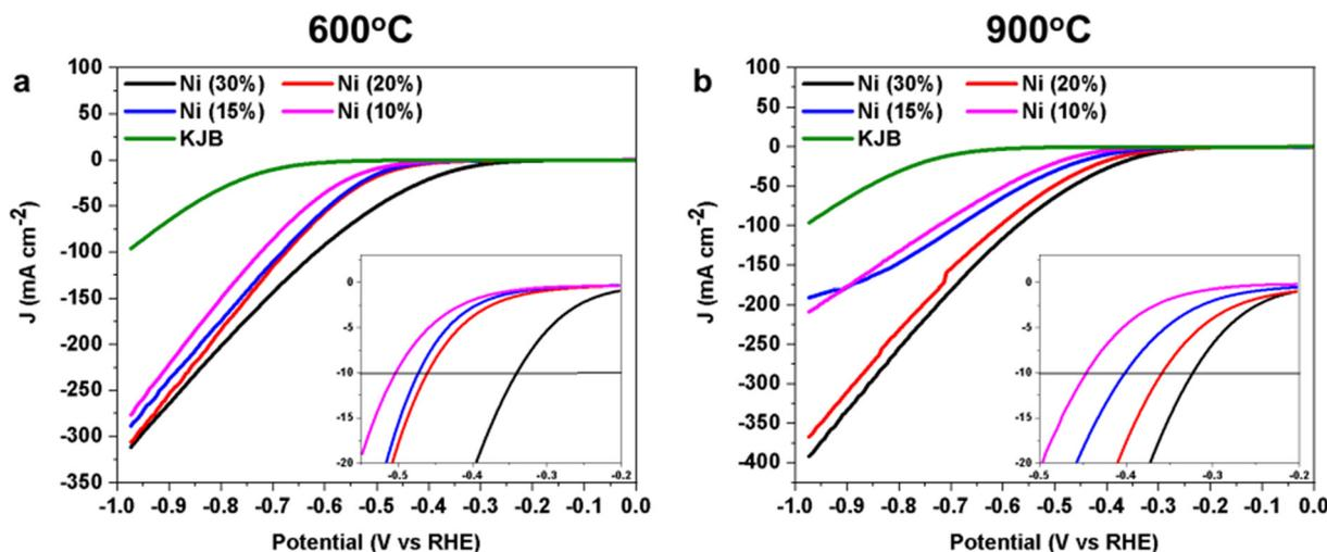
Fig. 9 The LSVs of the RDE measurement of KJB Ni-based electrocatalysts with different wt% of NiPc in their composition, and different thermal treatment temperatures of (a) 600 °C and (b) 900 °C in  $\text{N}_2$  saturated KOH (1 M) solution. The scan rate of  $5 \text{ mV s}^{-1}$  and a rotating disk speed of 1600 rpm were used for the measurements. The KJB carbon was measured as a control.
