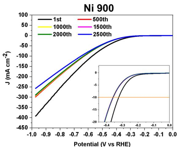
**Fig. 10** HER stability test (2500 cycles) on the Ni 900 electrocatalyst.
