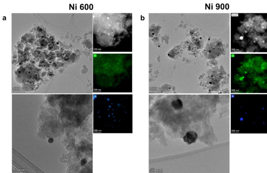
**Fig. 1** (a) TEM characterization of the Ni 600 °C and Ni 900 °C samples. For each sample, leftmost top image and bottom image report HRTEM characterization, while the rightmost column reports the STEM EDX mapping. (a) The Ni sample functionalized at 600 °C (Ni 600), and (b) the sample functionalized at 900 °C (Ni 900).
