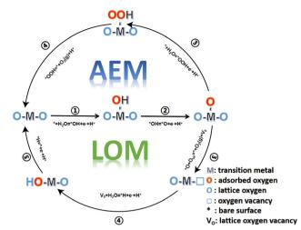
Fig. 2 Adsorbate evolving mechanism (AEM) and lattice oxygen mechanism (LOM)
