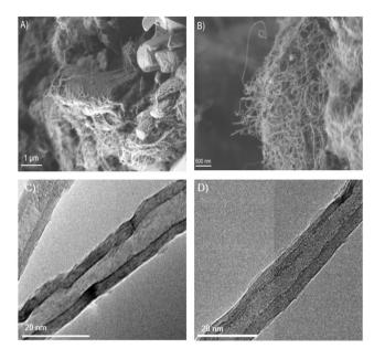
Fig. 14 Top row: Representative SEM images of product obtained by electrolyzing ( $Li_{0.62}K_{0.38}$ )<sub>2</sub>CO<sub>3</sub> + 13 mol% LiOH with 8 wt% LDPE at 14.2k× magnification (A) and 20.2k× (B). Bottom row: Representative TEM images of product obtained by electrolyzing  $(Li_{0.62}K_{0.38})_2CO_3 + 13$  mol% LiOH with 8 wt% LDPE (C) and the same with 8 wt% seaweed (D), confirming multiwalled carbon nanotubes.
