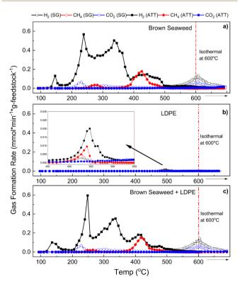
Fig. 6 Kinetic data for gas evolution of the main reaction gases, H<sub>2</sub>, CH<sub>4</sub>, and CO2, produced during the thermochemical steam gasification (SG) and alkaline thermal treatment (ATT) of BS (a), LDPE (b), and a 50:50 mixture of BS and LDPE (c). Open circles represent the SG reaction kinetic data whereas closed circles represent the ATT reaction kinetic data. Kinetic data are expressed as gas formation rate per minute per gram (mmol min $^{-1}$ a feedstock $^{-1}$ ).
