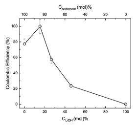
Fig. 13 Effect of initial LiOH content ( $C_{LiOH}$ , mol%) and initial carbonate content ( $C_{carbonate}$ , mol%) of the  $Li_2CO_3/K_2CO_3/LiOH$  electrolyte on the Coulombic efficiency of CO<sub>2</sub> electrosplitting process at 500 °C. The electrolyte Li<sub>2</sub>CO<sub>3</sub>/K<sub>2</sub>CO<sub>3</sub> mol ratio was set at eutectic 1.63 throughout.51
