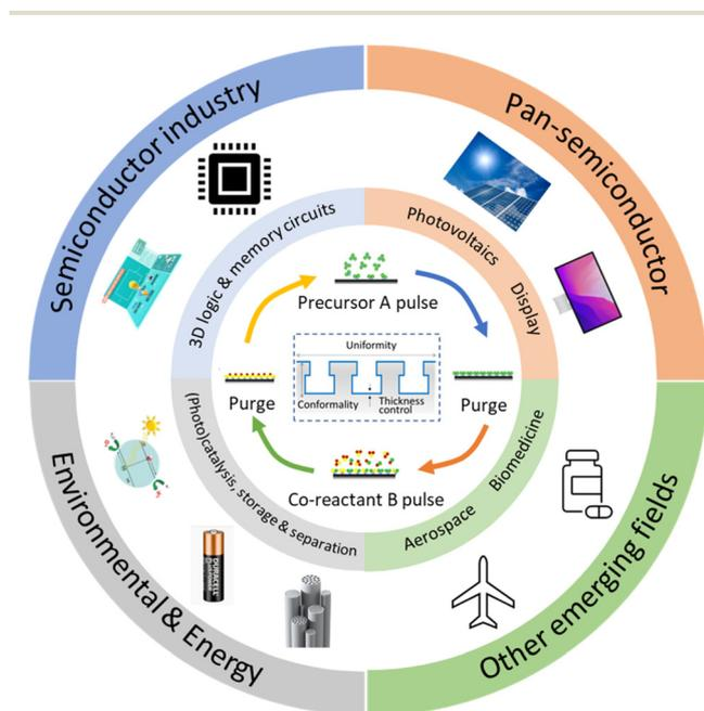
Fig. 1 Applications of ALD in the conventional semiconductor industry and other new emerging fields. Adapted from Zhang *et al.*<sup>9</sup>
