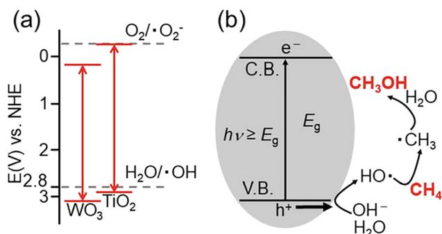
Fig. 9 Typical photocatalytic partial oxidation of methane to methanol mechanism catalyzed by metal oxide. (a) Redox potentials of WO<sub>3</sub> and TiO<sub>2</sub>. (b) Mechanism of the conversion of CH<sub>4</sub> to CH<sub>3</sub>OH by photocatalytic reaction. Adapted with permission from ref. 84 under the terms of the CC BY 3.0 license.
