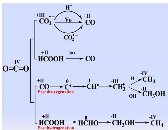
Fig. 4 Proposal of the reaction pathways for forming CO, CH<sub>4</sub>, and CH<sub>3</sub>OH in the photocatalytic CO<sub>2</sub> reduction. Reproduced with permission from ref. 52 under the terms of the CC BY 4.0 license.
