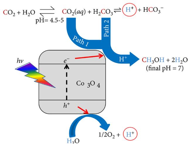
Fig. 6 Mechanism for the photocatalytic reduction of aqueous CO<sub>2</sub> in the presence of Co<sub>3</sub>O<sub>4</sub>. Reproduced with permission from ref. 60 under the terms of the CC BY 4.0 license.
