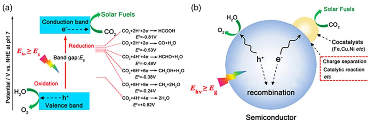
Fig. 11 Schematic diagram of the photocatalytic reduction of  $\text{CO}_2$  to solar fuels. (a) Energy diagram for  $\text{CO}_2$  reduction and water oxidation on a semiconductor. (b) Schematic of the photocatalytic reaction process and influencing factors. Reproduced with permission from ref. 92 under the terms of the CC BY-NC-ND 4.0 license.
