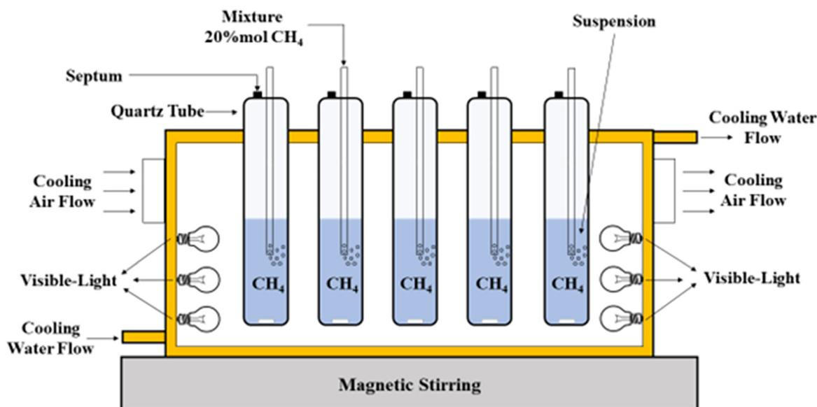
**Fig. 7** Experimental setup for the photocatalytic partial oxidation of CH<sub>4</sub> to CH<sub>3</sub>OH. Reproduced with permission from ref. 81.
