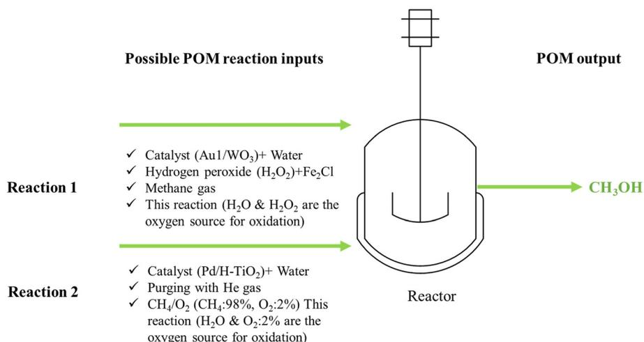
Fig. 8 Possible POM inputs with different reaction conditions.
