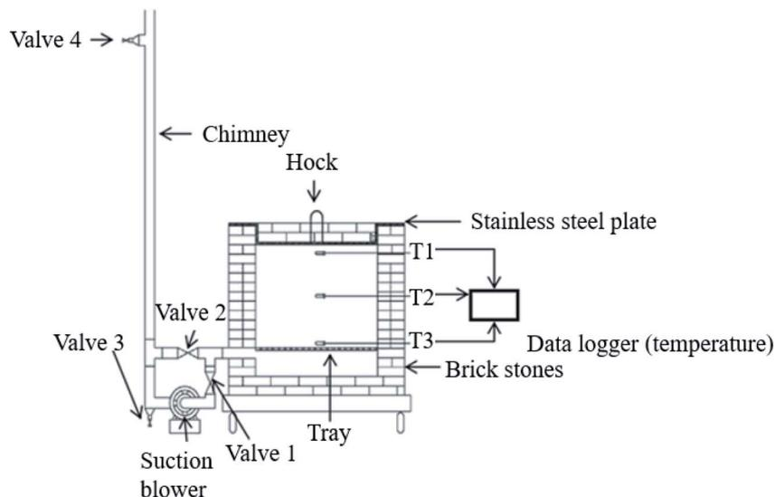
Fig. 5 A self-sustained reactor for industrial-scale biochar production.
