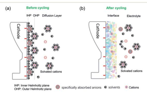
Fig. 8 A schematic diagram of the cathode-electrolyte interface before and after cycling and the formed CEI after cycling. (a) The ions and solvents will be specifically absorbed on the inner Helmholtz plane (IHP) before cycling. (b) The specific species of the IHP and the solvated groups become oxidized or otherwise decomposed during cycling, along with the disappearance of the IHP. Reproduced under CC-BY licence from ref. 103.
