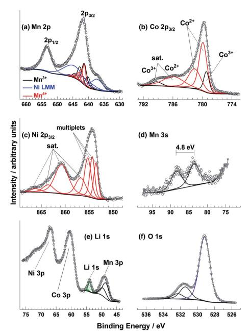
Fig. 7 Mn 2p, Co 2p, Ni 2p, Mn 3s, Li 1s, and O 1s XPS spectra for a radio frequency magnetron sputter deposited Li–Ni–Mn–Co–O thin film sample. Reprinted with permission from ref. 90 Copyright 2017 John Wiley & Sons, Ltd.
