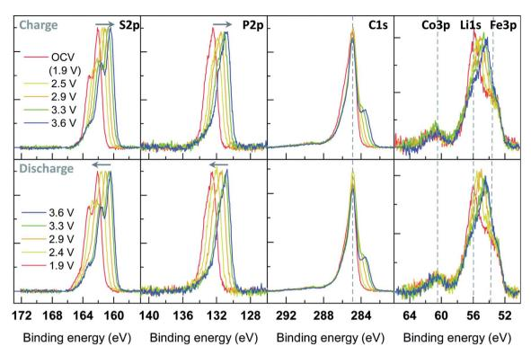
Fig. 29 Operando XPS experimental results during potentiostatic measurement of a working electrode made of 45 wt% LCO, 50 wt% amorphous  $(\text{Li}_2\text{S})_3 - \text{P}_2\text{S}_5$  and 5 wt% VGCF cycled vs.  $\text{InLi}_x$ . Reprinted from ref. 182.
