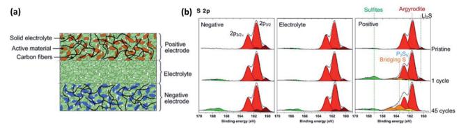
Fig. 23 (a) Scheme of a typical all-solid-state cell. (b) XPS measurements of the different parts of all-solid-state cell after different number of electrochemical cycling. Reprinted from ref. 177, with permission from Elsevier.
