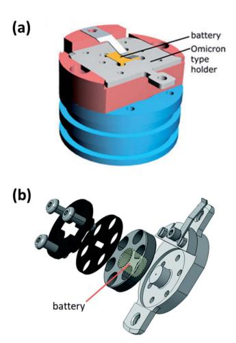
Fig. 28 Different set-ups used for operando XPS. (a) Sample holder for micro-batteries. Reprinted from ref. 200, with permission from AIP Publishing. (b) Sample holder for bulk ASSBs. Reprinted from ref. 182.
