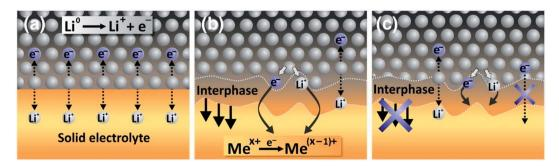
Fig. 22 Interphases in ASSBs. (a) The stable interphase. (b) The mixed conducting interphase (MCI). (c) The solid electrolyte interphase (SEI). Reprinted from ref. 175, with permission from Elsevier.
