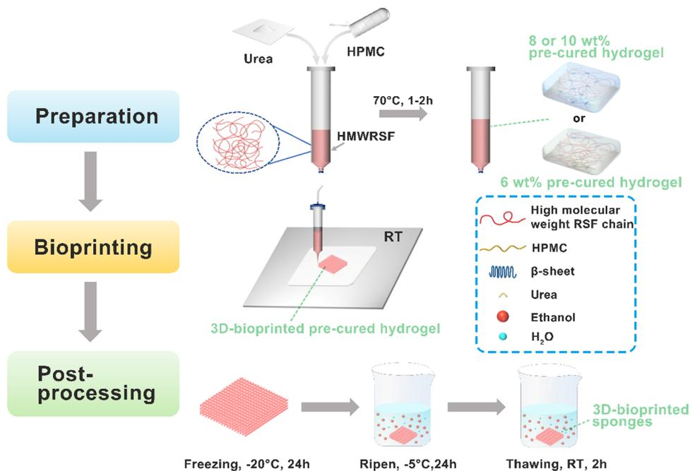
**Fig. 1** Schematic illustration of the preparation, bioprinting, and post-processing procedure of HMWRSF-based pre-cured hydrogels. HMWRSF: high-molecular-weight regenerated silk fibroin, HPMC: hydroxypropyl methylcellulose, and RT: room temperature. Urea was not introduced for a 6 wt% pre-cured hydrogel.
