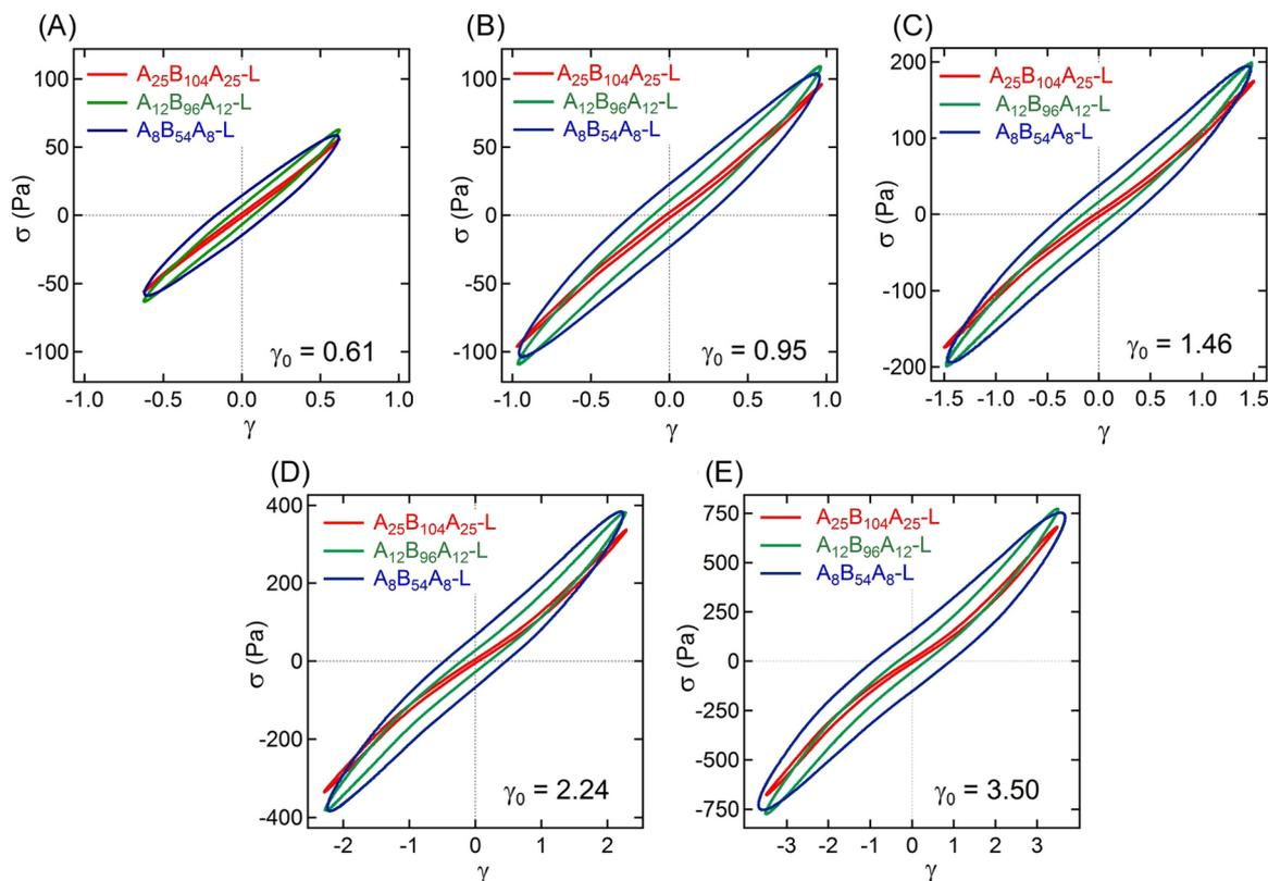
Fig. 4 Lissajous plots for  $A_{25}B_{104}A_{25}$ -L,  $A_{12}B_{96}A_{12}$ -L, and  $A_8B_{54}A_8$ -L obtained from amplitude sweep experiments displaying the shear stress ( $\sigma$ ) vs. intracycle strain ( $\gamma$ ) at  $\gamma_0 \approx$  (A) 0.61, (B) 0.95, (C) 1.46, (D) 2.24, and (E) 3.50. The experiments were performed using  $\omega = 1 \text{ rad s}^{-1}$ .
