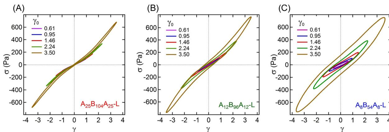
Fig. 3 Lissajous plots obtained from amplitude sweep experiments displaying the shear stress ( $\sigma$ ) vs. intracycle strain ( $\gamma$ ) for (A) A<sub>25</sub>B<sub>104</sub>A<sub>25</sub>-L, (B) A<sub>12</sub>B<sub>96</sub>A<sub>12</sub>-L, and (C) A<sub>8</sub>B<sub>54</sub>A<sub>8</sub>-L for  $\gamma_0 \approx 0.61, 0.95, 1.46, 2.24$ , and  $3.50$ . The experiments were performed using oscillatory frequency ( $\omega$ ) of 1 rad s<sup>-1</sup>.
