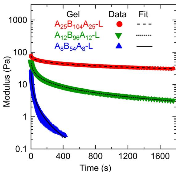
Fig. 6 Shear modulus ( $G(t)$ ) as a function of time ( $t$ ) for  $A_{25}B_{104}A_{25}$ -L,  $A_{12}B_{96}A_{12}$ -L, and  $A_8B_{54}A_8$ -L obtained from stress-relaxation experiments for a step-strain of  $\gamma_0 = 0.01$  at  $\approx 27^\circ\text{C}$ . The lines represent the fitting of the stretched-exponential model (eqn (3)).
