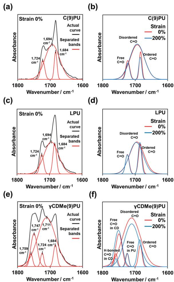
Fig. 5 Actual FT-IR spectra and separated bands after peak deconvolution of C(9)PU (a), LPU (c), and  $\gamma$ CDMe(9)PU (e) before tensile stretching. Changes in the separated bands of C(9)PU (b), LPU (d), and  $\gamma$ CDMe(9)PU (f) during tensile stretching from 0% to 200% strain.
