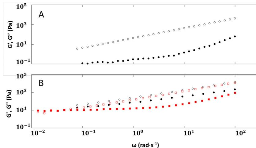
Fig. 6 Moduli versus angular frequency sweeps ( $\omega$ ) of imidazolium ionomers with hexyldithiocarbamate and octadecyldithiocarbamate anions: (A) **2–6** ( $\bullet$  =  $G'$ ,  $\circ$  =  $G''$ ), at 25 °C and 1% strain; (B) **2–18** ( $\bullet$  =  $G'$ ,  $\circ$  =  $G''$ ) at 40 °C and 0.5% strain and **2–18** ( $\blacksquare$  =  $G'$ ,  $\square$  =  $G''$ ) at 50 °C and 0.5% strain.
