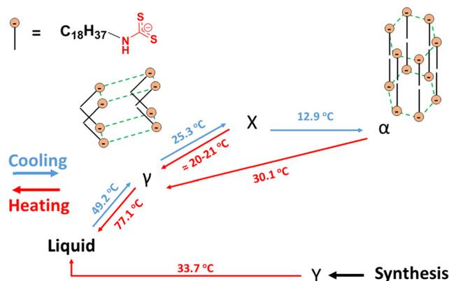
**Fig. 4** Cartoon representations of the proposed packing arrangements of the anions and designations of transition types and their peak temperatures for morphs of the 2–18 ionomer, based on DSC and PXRD data. ‘Synthesis’ refers to the initially isolated material from a reaction mixture in which the solvent was chloroform.
