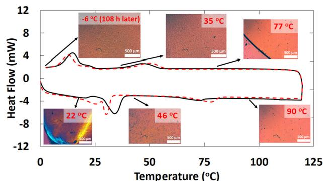
**Fig. 3** DSC thermogram of 2–18 for the first (black) and second heating-cooling cycle (red dashed). Polarized optical micrographs taken during the first heating and cooling are shown at the indicated temperatures.
