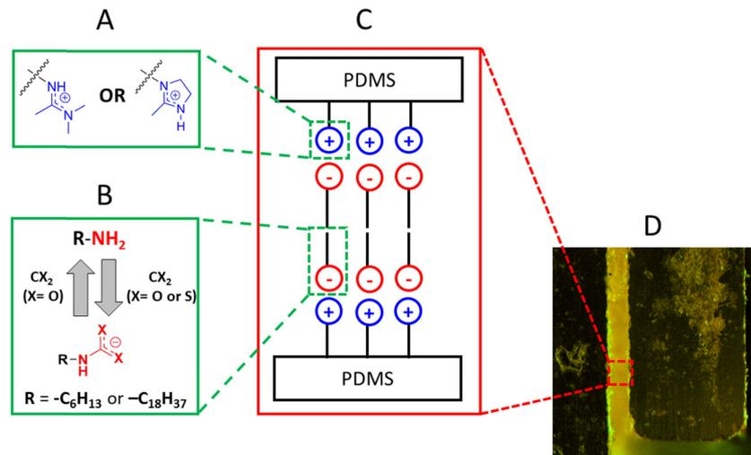
Fig. 1 (A) Amidinium (left) and imidazolium (right) groups; (B) choosing the triatomic  $CX_2$  and alkyl chain length; (C) ionic (coulombic) attractions among the ionic centers along the chains and van der Waals (dispersive) interactions along the alkyl chains of the anions; and (D) one of the resulting materials applied as an adhesive to borosilicate glass surfaces.
