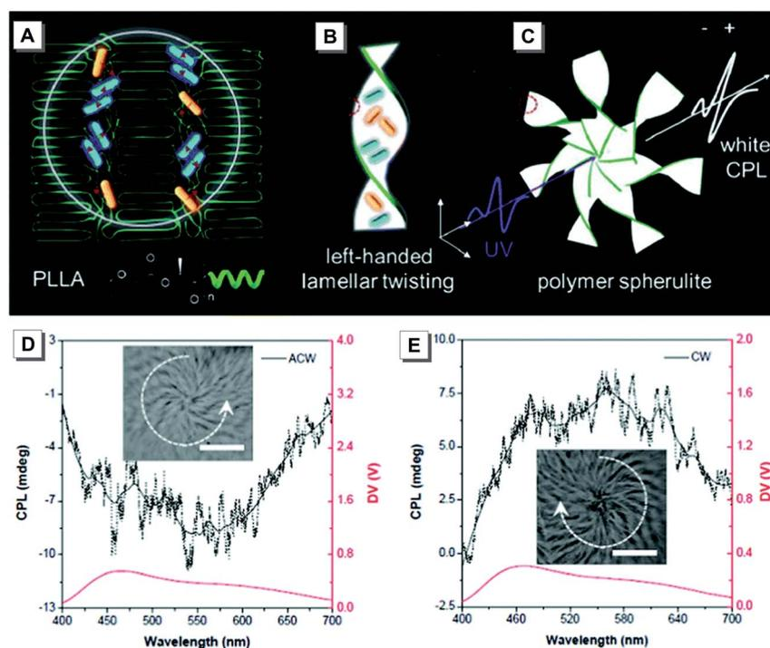
Fig. 18 (A) White emission from **43** packed in the amorphous region between polymer crystalline lamellae. (B and C) The formation of 3D spiral banded spherulites and the generation of CPL. (D and E) The CPL spectrum switching by the inversion of the P-PLLA film. Insets: Bright-field images of 3D spiral patterns of the spherulites from two different sides. Adapted from ref. 44 with permission. Copyright 2019 the Royal Society of Chemistry.
