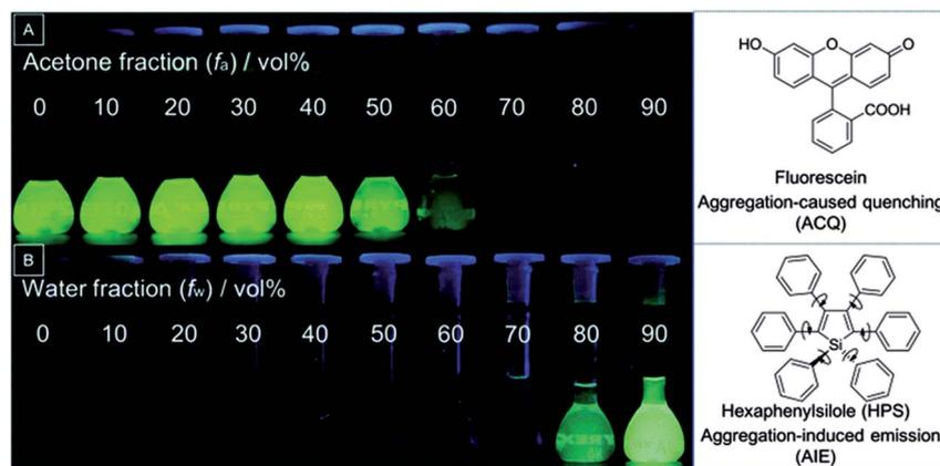
Fig. 1 Fluorescence images of (A) fluorescein ( $1.5 \times 10^{-2}$  M) in a mixed solvent of water and acetone with different fractions of acetone ( $f_a$ ), and (B) hexaphenylsilole (HPS;  $1.0 \times 10^{-2}$  M) in a mixed solvent of THF and water with different fractions of water ( $f_w$ ). Reproduced from ref. 34 with permission. Copyright 2015 the Royal Society of Chemistry.
