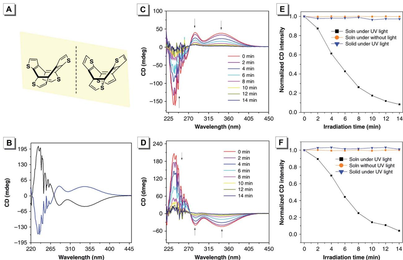
Fig. 17 (A) Molecular structures and (B) CD spectra of the two enantiomers of **37** in THF solution. (C and D) The changes of CD spectra of the two enantiomers in THF solution under UV irradiation for different times. (E and F) Time-dependent CD spectral change profiles of the two enantiomers in THF solution and the solid state with or without UV irradiation. Adapted from ref. 42 with permission. Copyright 2019 Nature Publishing Group.
