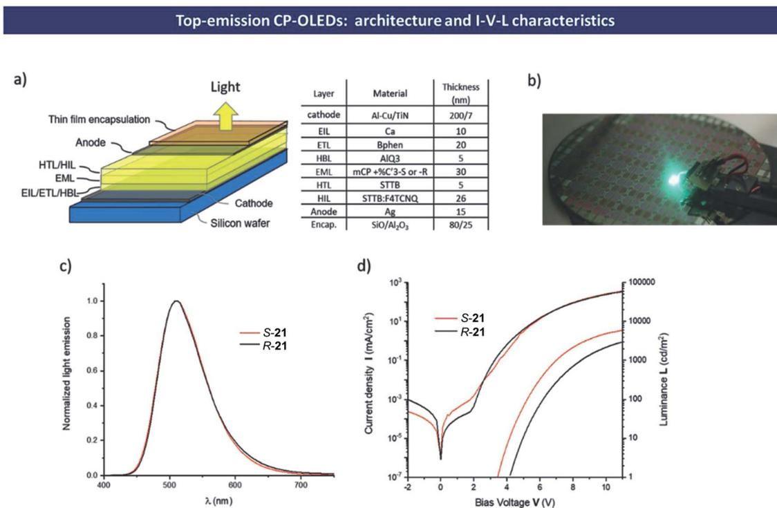
Fig. 21 (a) Device structure of a top-emission CP-OLED built from a typical thin film stacked with *R*-21 and *S*-21 chiral dopants. (b) The test of an individual CPOLED in 8 inch wafer level-processed CP-OLEDs. (c) Light emission spectrum of CP-OLEDs integrating either *S*-21 or *R*-21 chiral dopants; (d) corresponding *I*–*V*–*L* characteristics. Adapted from ref. 69 with permission. Copyright 2020 Wiley-VCH.
